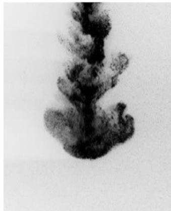
Figure 1-3: Image of sand jet passing through 4mm nozzle diameter in water.
