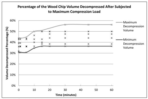
Figure 10: Graph showing the range of wood chip decompression over time.
