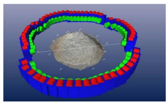
Figure 5: 3D model of the chip pile showing the location of all the camera locations.
