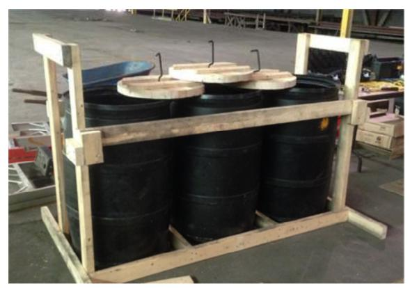
Figure 1: Three 44-imperial gallon barrels used for compression and decompression testing.
