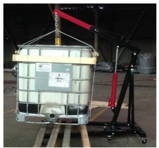
Figure 2: One cubic meter container used for measuring the wood chips on a small scale pile.
