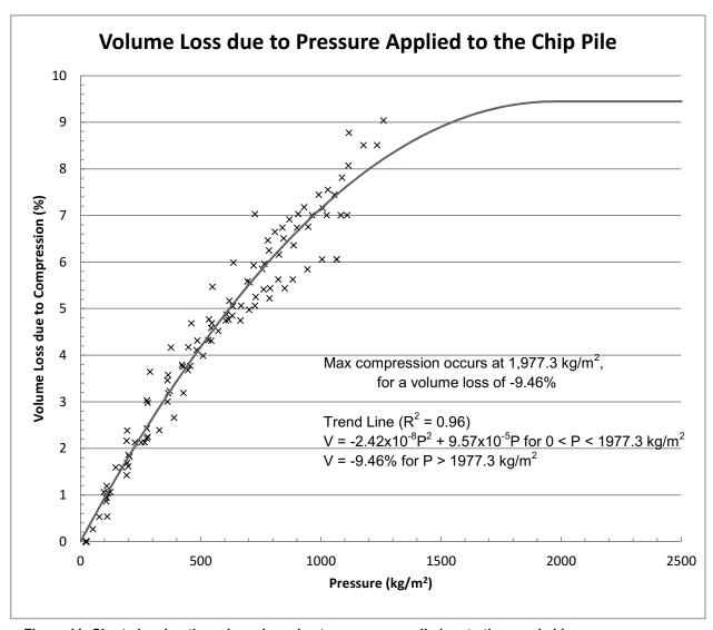
Figure 11: Chart showing the volume loss due to pressure applied on to the wood chips.
