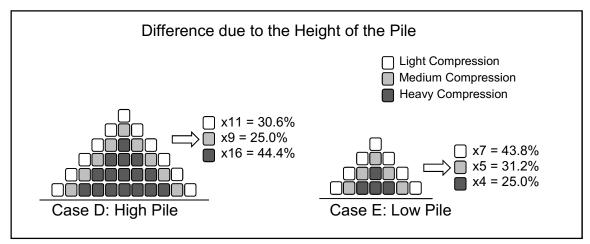
Figure 17: Showing the different varying densities of wood chips as the pile changes in height.
