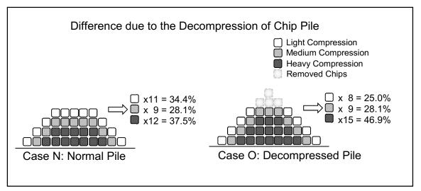
Figure 21: Showing the different varying densities of wood chips as one pile goes through decompression while the other pile is formed normally.
