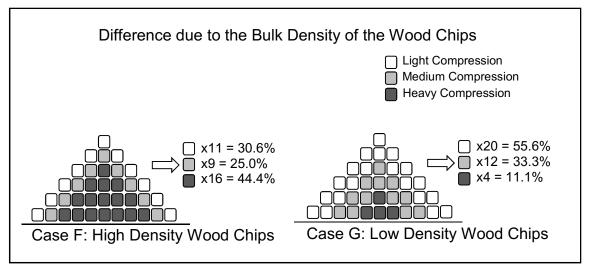
Figure 18: Showing the different varying densities of wood chips as the bulk density changes.
