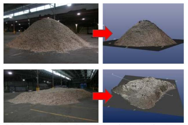
Figure 6: Transition from photo image to 3D model on the computer for both conical and flattened piles.
