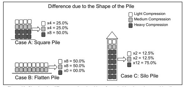
Figure 16: Showing the different varying densities of wood chips throughout a chip pile as shape varies from a square pile, a flattened pile, and a tall pile in a silo.
