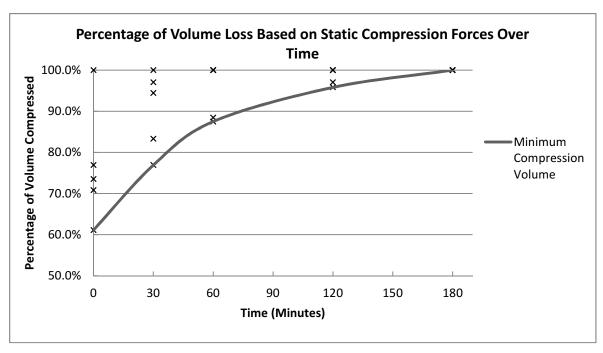
Figure 9: Graph showing the percentage of volume loss due to static compression applied over time.
