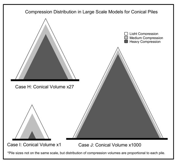
Figure 19: Graphic models of compression distribution in the predicted conical piles of Table 6: Chart showing the difference between CCC and mill estimates for both conical and flattened pile
