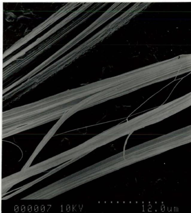
Figure 3.3. SEM micrograph showing filamentous bundle structure.
