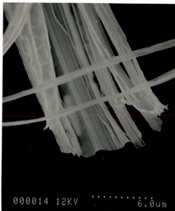
Figure 3.4. SEM micrograph showing striated, sheet-like structure of crystals.
