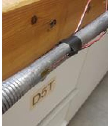
Figure 15 Anchor Rod Strain Gauge Assembly
