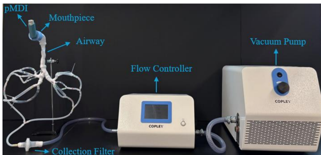
Fig. 3-6: Experimental setup includes Salbutamol HFA pMDI, male airway replica extracted from CT-scan images, flow controller, and vacuum pump.
