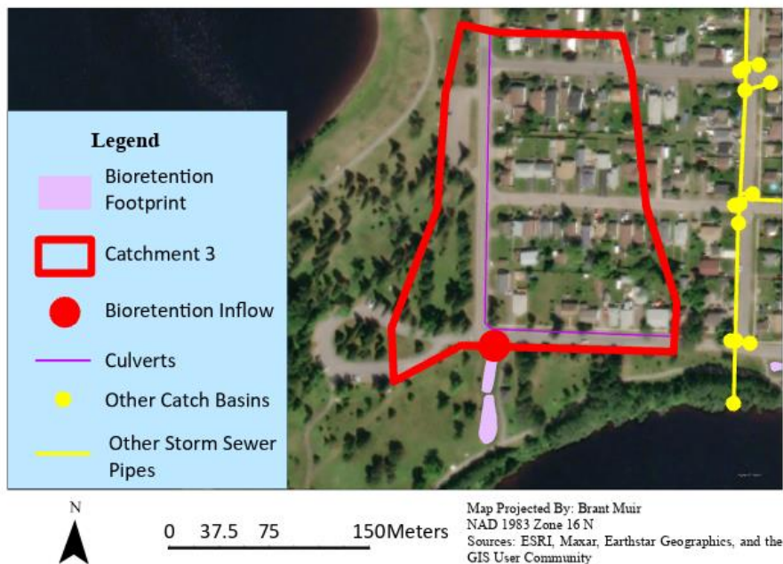
Neighboring Stormwater Infrastructure at Bioretention System 3
