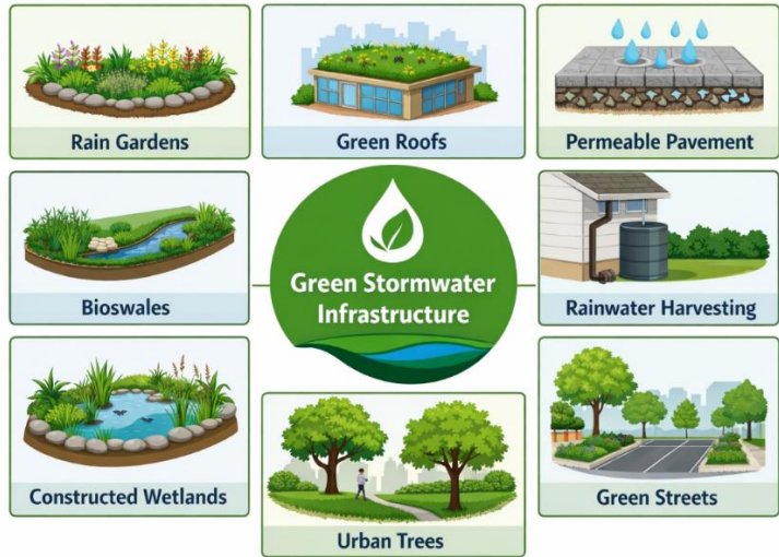
Figure 2-2 Common forms of green stormwater infrastructure for stormwater quantity and quality management.
