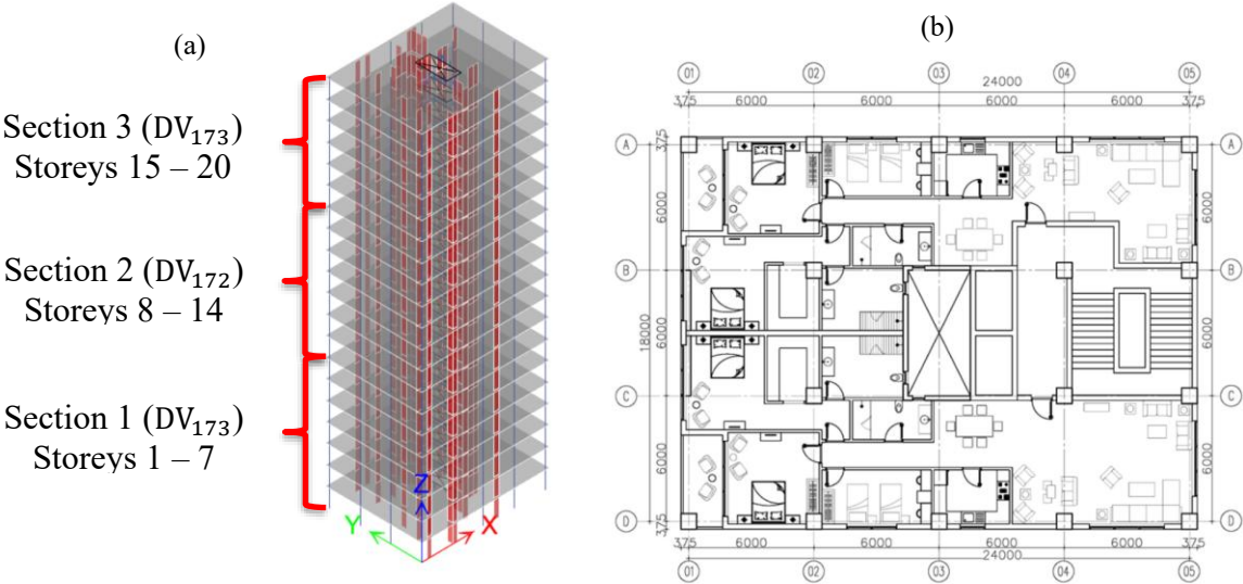
Figure 4.3 – Study building a) isometric conceptual view b) plan view with architectural details
