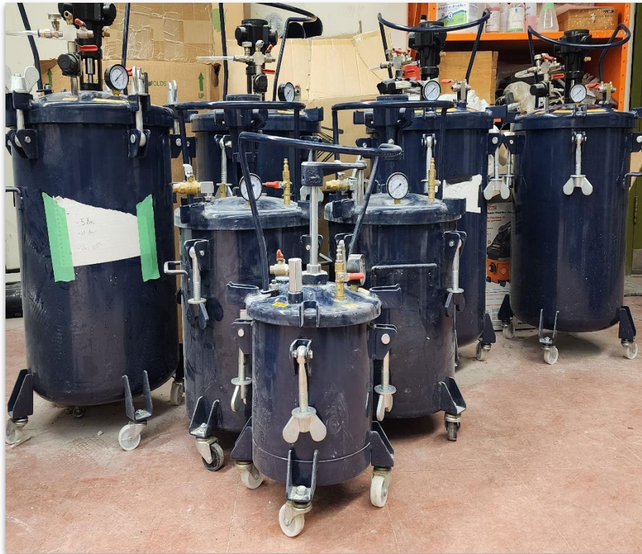
Figure 3.2: Collection of Pressure Tanks
