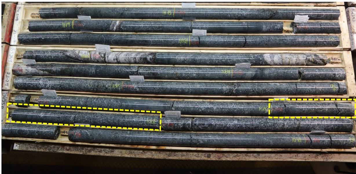
Figure 3.2 – Vari-textured gabbro from sample 22 711 gc 001 selected for U–Pb geochronology (1087–1088 m). Dashed yellow boxes highlight the intervals chosen for analysis.
