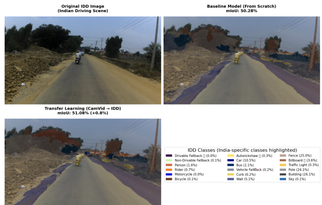
Figure 13. Prediction overlays on IDD dataset. (Top image): baseline prediction; (bottom image): transfer learning from CamVid. Improved detection of road area, vegetation, and person classes.
