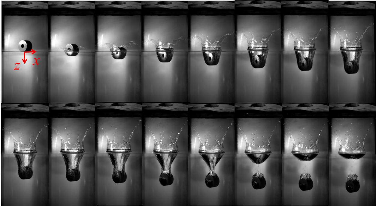
Figure 5.4: Time history images of oblique 45^\circ view of a free-falling annular disk in stagnant water. The hole diameter ratio, density ratio, and aspect ratio of the test are d_h/D = 0.33 , \rho_d/\rho_w = 1.14 , D/h = 1.5 , respectively. The time interval between each image is \Delta t = 0.01 s.
