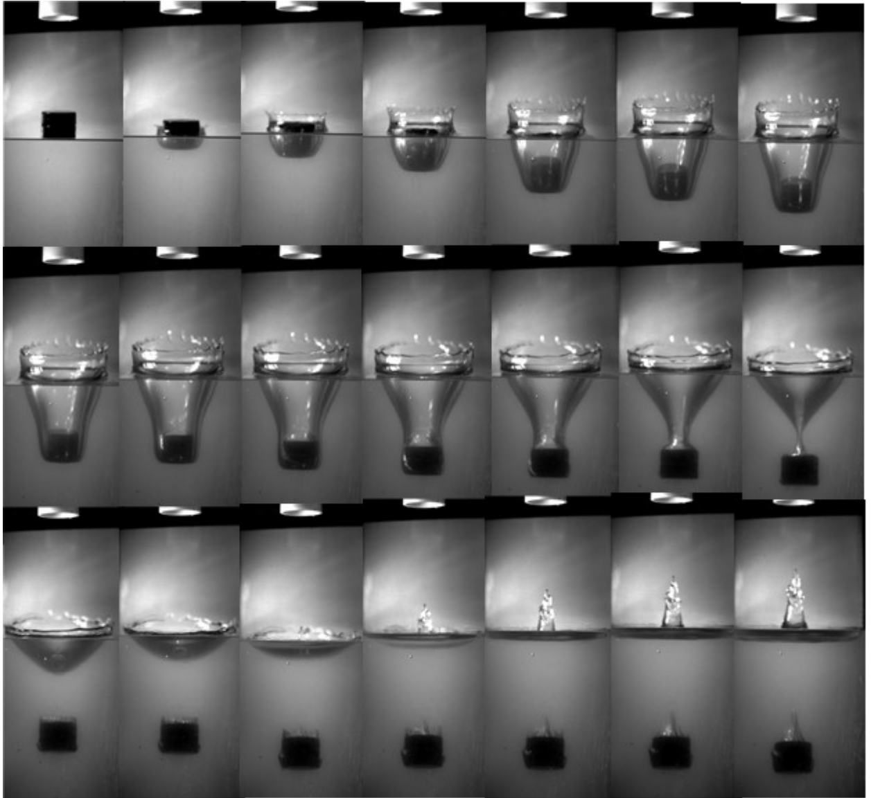
Figure 2.7: Time history images of a free-falling disk with a density ratio of 1.45 and an aspect ratio of 1.5 in a stagnant fluid mixture with 0.3 wt. % PAM concentration. The time interval between each image is 0.01 seconds.
