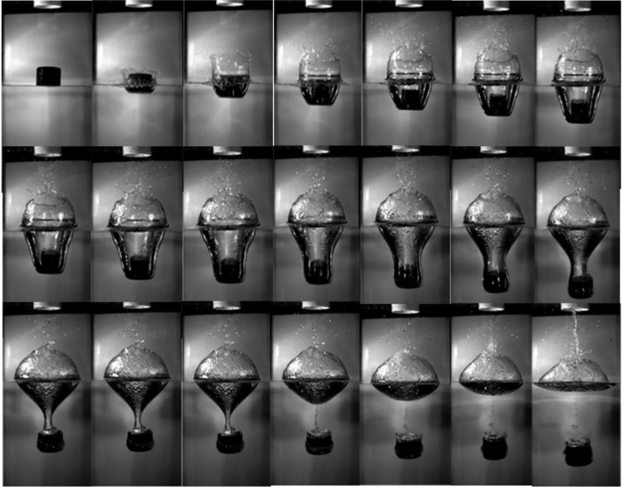
Figure 2.4: Time history images of a free-falling disk in stagnant water with a density ratio of 1.48 and an aspect ratio of 1.5. The time interval between each image is 0.01 seconds.
