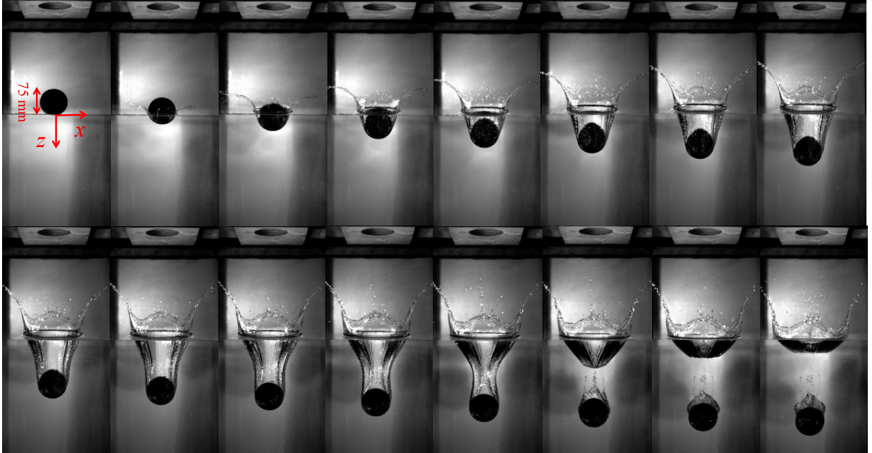
Figure 5.3: Time history images of frontal view for a free-falling solid disk in stagnant water. The density ratio and aspect ratio of the disk is \rho_d/\rho_w = 1.48 , D/h = 1.5 . The time interval between each image is \Delta t = 0.01 s.
