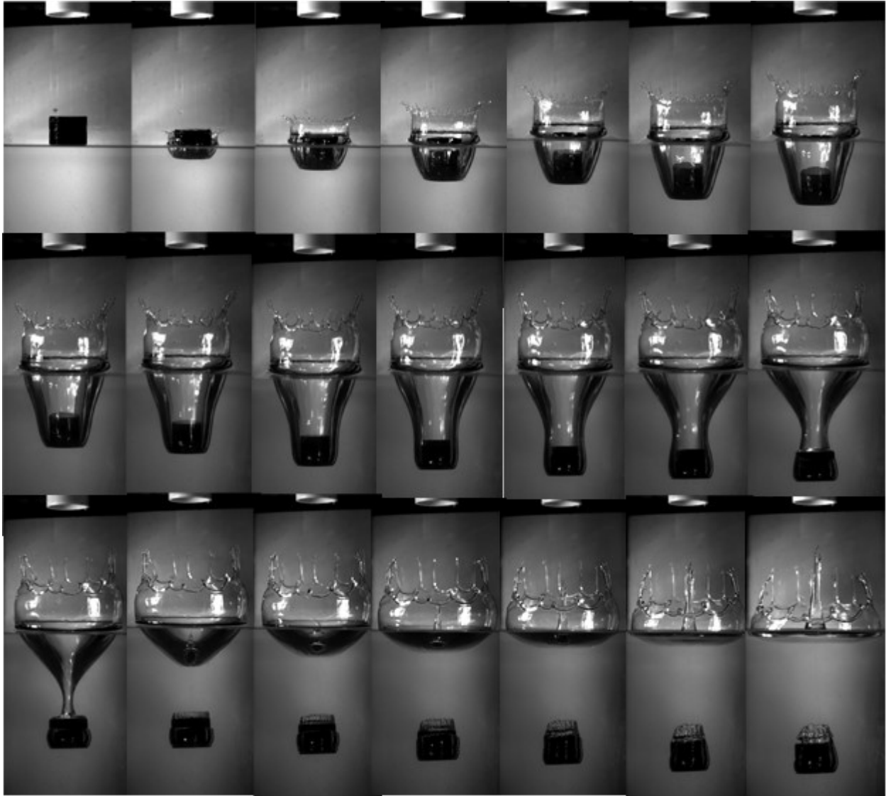
Figure 2.6: Time history images of a free-falling disk with a density ratio of 1.45 and an aspect ratio of 1.5 in a stagnant fluid mixture with 0.1 wt. % PAM concentration. The time interval between each image is 0.01 seconds.
