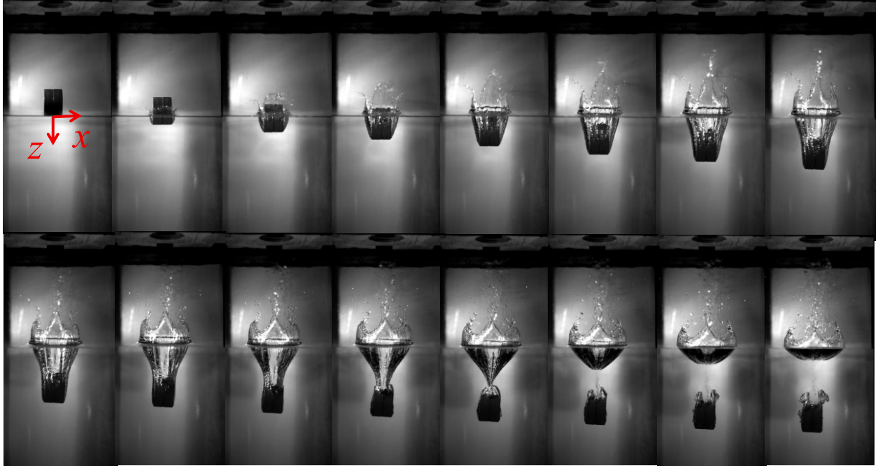
Figure 5.5: Time history images of side view of a free-falling annular disk in stagnant water. The hole diameter ratio, density ratio, and aspect ratio of the test are d_h/D = 0.33 , \rho_d/\rho_w = 1.14 , D/h = 1.5 , respectively. The time interval between each image is \Delta t = 0.01 s.
