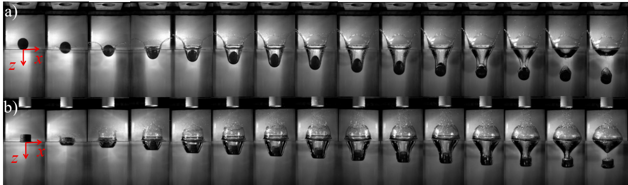
Figure 5.7: A comparison between the edge-on and face-on entry of solid disk impacting in stagnant water. Both disks have a density ratio of \rho_d/\rho_w = 1.14 and an aspect ratio of D/h = 1.5 . The
