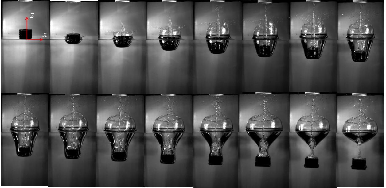
Figure 4.2: Time history images of a free-falling annular disk in stagnant water. The opening diameter ratio of the cylinder is d_h/D = 0.20 , the density ratio is \rho_d/\rho_w = 1.48 , and the aspect ratio is D/h = 1.5 . The time interval between each image is 0.01 seconds.
