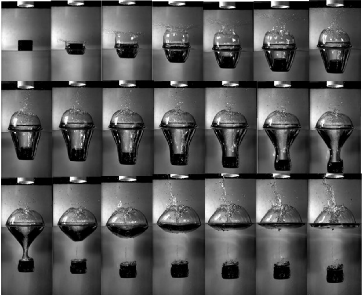
Figure 2.5: Time history images of a free-falling disk with a density ratio of 1.45 and an aspect ratio of 1.5 in a stagnant fluid mixture with 0.01 wt. % PAM concentration. The time interval between each image is 0.01 seconds.
