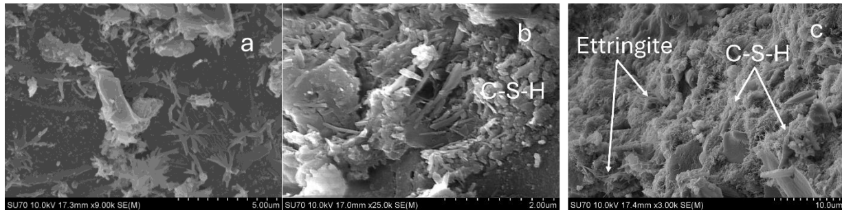
Figure 3.13: SEM images of a) BFA 15%, b) SL 30%, c) GP 30%
