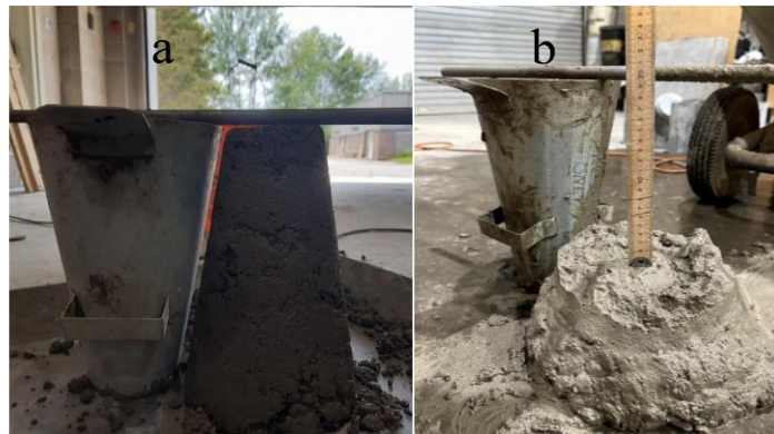
Figure 4.9: a) Mix No.11 (7.5% SH, 10% GP, 15% BA) zero slump b) Mix No.7 (7.5% SR, 10% GP, 7.5% BFA) 192 mm slump
