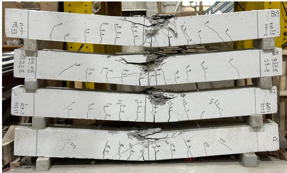
Figure 6.14 Concrete beam specimens after test, showing compression failure
