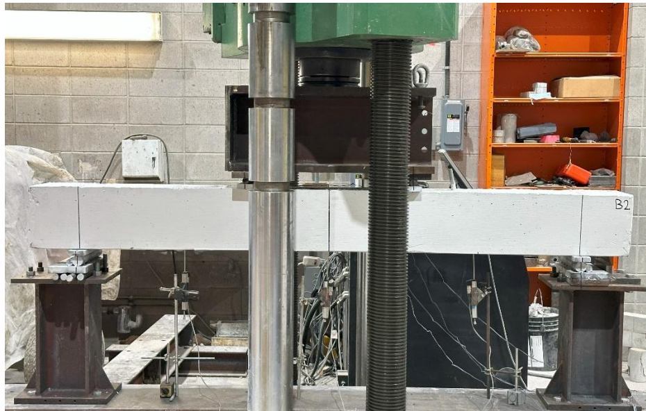
Figure 6.11: Four-point flexural beam setup
