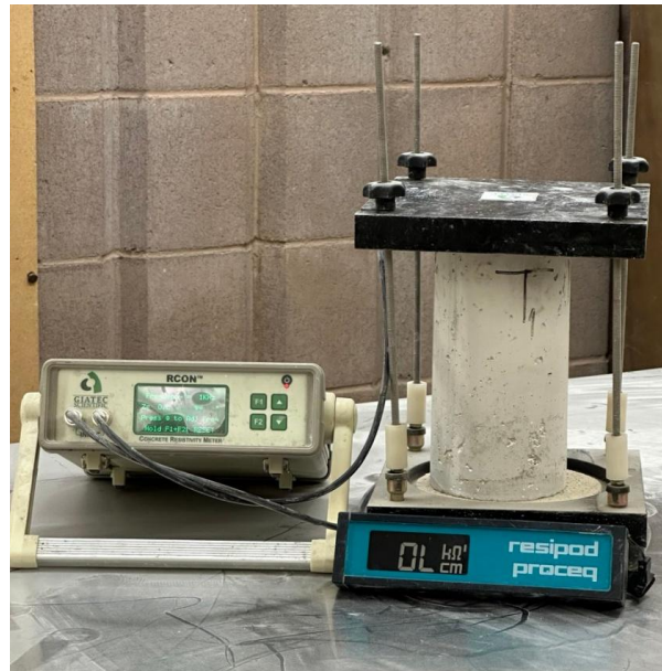
Figure 2.8: Bulk and surface electrical resistivity instruments
