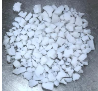
Figure 5-10: Laponite hydrogel after dried up at 100°C for 24 hours in a temperature-controlled oven
