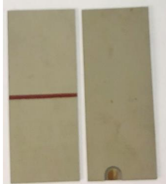
Figure 6-4: Bender Elements manufactured by Piezo.com, Division of Mide Technology, Woburn, MA, United States.
