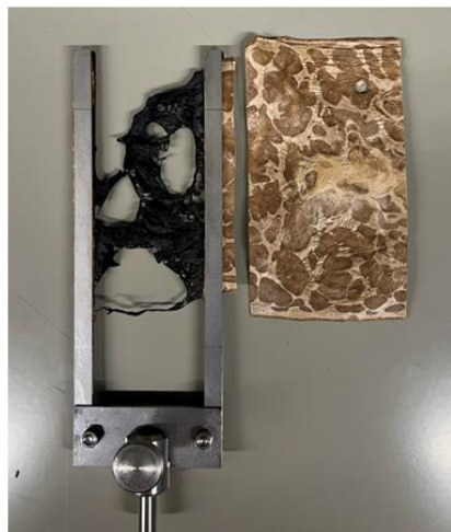
Figure S3.8. PLA film mixed with PK17, before and after LOI test.
