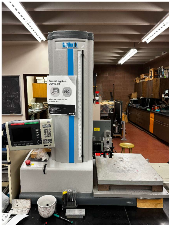
Figure C.1 – The Chatillon Force Tester and AMTI force plate
