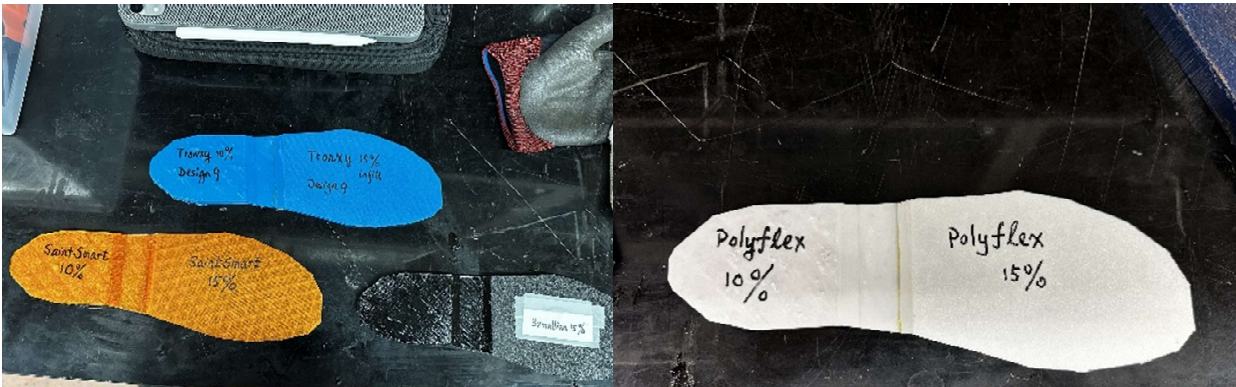
Figure 4.10: TPUs Used for Insoles
