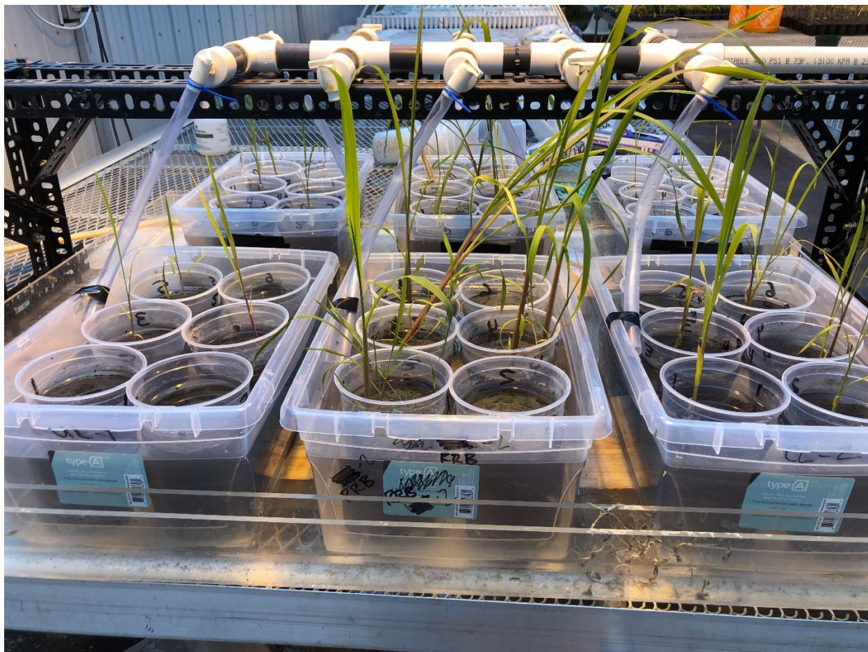
Figure 2.2. August 21, 2019. Microcosm-scale WR sediment exposure chambers. Left to Right: six replicates of Unnamed Lake; Rat River Bay, and Cleaver Lake. Six additional replicate exposures of each sediment were placed on the opposing side of the water bath.
