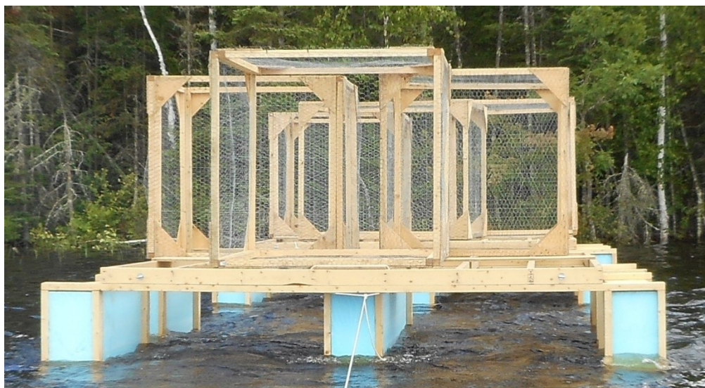
Figure 3.5. Configuration of raft assemblies used at the Seine River deployment location. Wire-mesh encased quadrats were attached between the Styrofoam floats.
