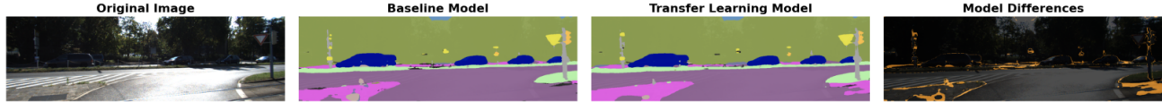
Figure 4. Qualitative comparison of baseline vs. transfer learning models on KITTI. From left to right: Original image, baseline model prediction, transfer learning model prediction, and visualization of differences between models. The last column highlights areas where transfer learning provides improved boundary precision and class recognition (shown in brighter regions).
