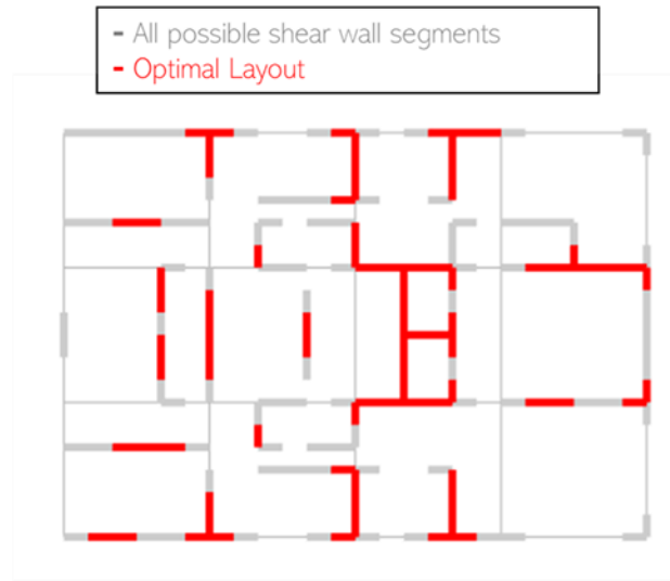
Fig. 2-23 Optimal shear wall layout of optimization Problem-4
