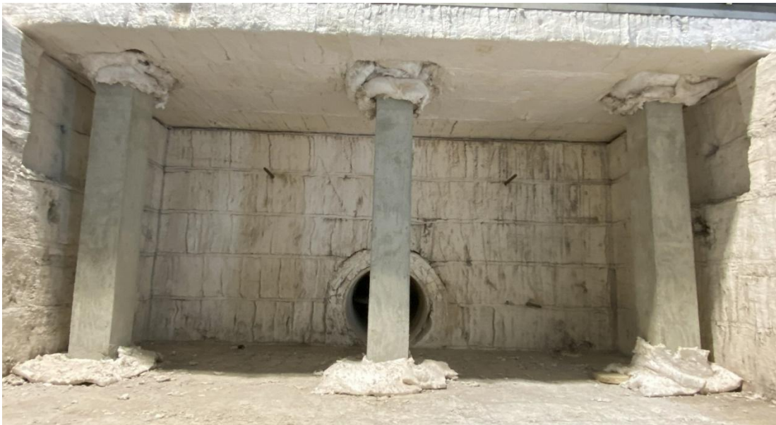
Figure 2.3 Furnace setup prior to Fire Test 3, showing a typical three-column configuration and thermal insulation around the column ends.
