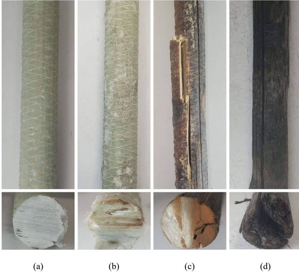
Figure 2.8 Condition of GFRP reinforcement before and after exposure. a) Control GFRP bar with no exposure and no test, b) GFRP bar extracted from ambient-temperature specimen, c) GFRP bar extracted from specimen exposed to 1-hour standard fire, and d) GFRP bar extracted from specimen exposed to 2-hour standard fire
