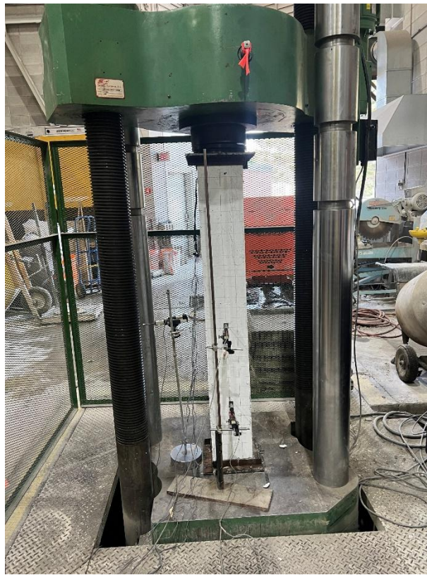
Figure 2.4 Typical axial compression test setup for a slender column in the 500-kip UTM.
