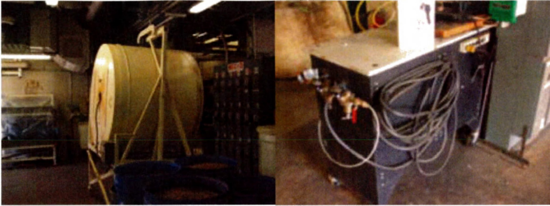
Figure 14. Diagram of Small Batch Blender (Left) and Atomized Resin Spraying System (Right).
