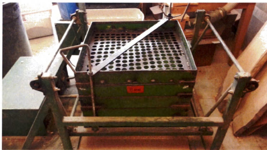
Figure 12. Diagram of Chip Screening Apparatus.
