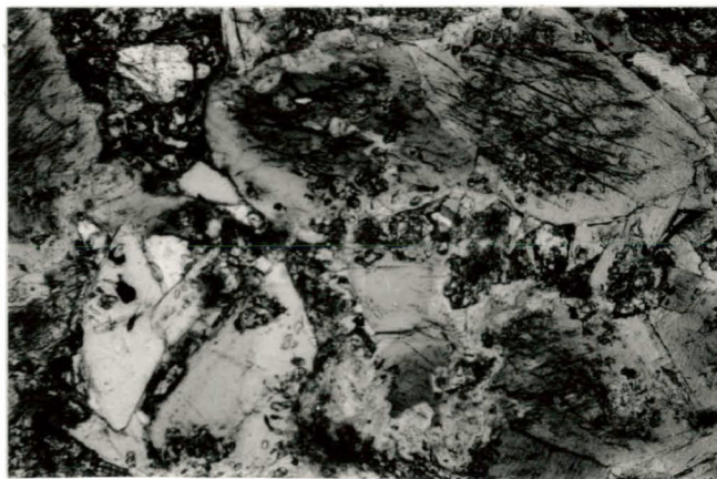
Figure 3.13: Weakly zoned hornblende within clinopyroxene hornblendite (FOV 2.7 mm). Sample AM-3-85, Mud Lake Intrusion.
