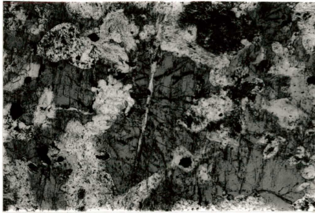
Figure 3.14: Actinolite/carbonate pseudomorphs after clinopyroxene enclosed in an oikocryst of hornblende (FOV 2.7 mm). Sample AM-4-85.
