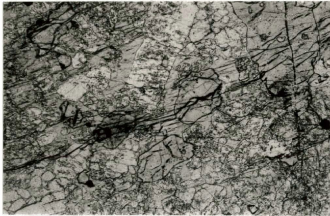
Figure 3.9: Olivine hornblende clinopyroxenite (FOV 2.7mm). Sample AK-12-86, Kawene Intrusion.
