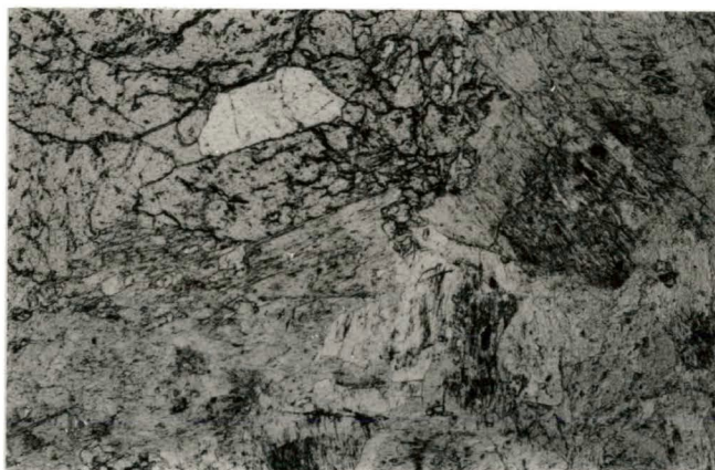
Figure 3.12: Clinopyroxene hornblendite (FOV 2.7 mm). Sample AK-49-86, Kawene Intrusion.
