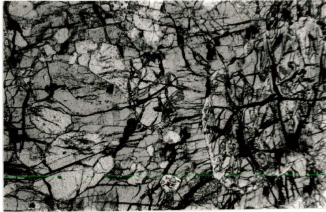
Figure 3.3: Hornblende wehrlite (Sample AK-40-86). Note intense fracturing of minerals surrounding serpentinized olivine (FOV 2.7 mm).
