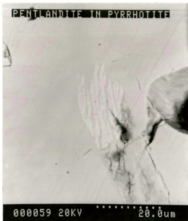
Figure 5.2c: Cluster of pentlandite exsolution flames within pyrrhotite. Sample #17, Drill Hole K-1-87.
