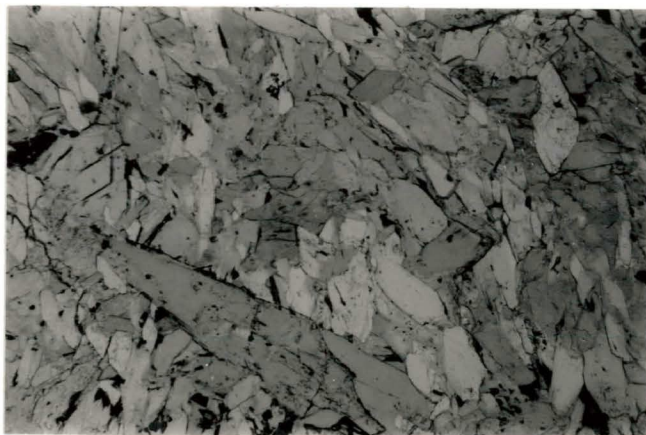
Figure 3.11: Slightly recrystallized hornblendite (FOV 2.7 mm). Sample AAb-10-85, Abiwin Intrusion.
