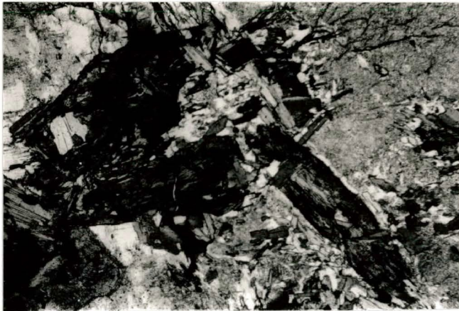
Figure 3.18: Cored hornblende grain within apatite (FOV 2.7 mm). Sample AML-6-85.
