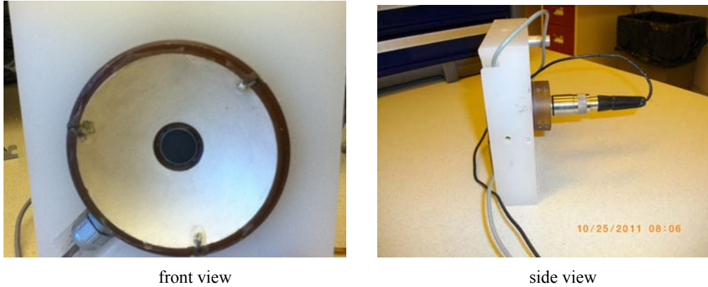
Figure 15. The front view and side view of the confocal of FUS transducer and imaging transducer. The focal length for both transducers is 60mm. and inner and outer diameters of the FUS transducer are 20 and 85 mm, respectively. The diameter of imaging transducer is 15.8mm
