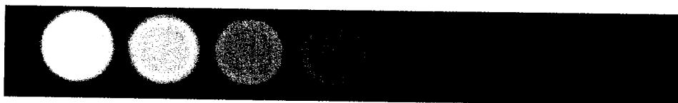
Figure 12: The effect due to the concentration of SPIO nanoparticles on MRI image. MRI output images corresponding to the first 7 data points. SPIO concentration increases from left to right.
