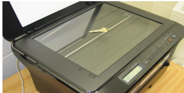
Figure 3.1 scanning the key using an open lid scanner
