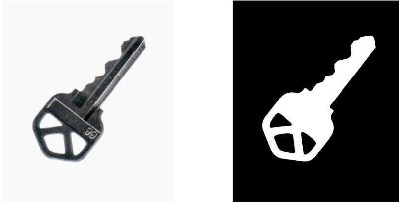
a b Figure 3.30 (a) Original color image. (b) Binary image after using filledBinary function
