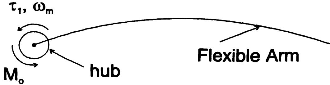
Figure 3.4. Positive direction of reaction torque, M_o at the hub caused by flexing of the arm due to applied torque \tau_1 .
