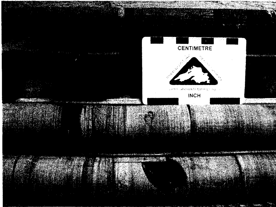
Fig.35. Coarsening and Thickening Upward Succession. A carbon-rich shale and siltstone interval (upper two rows). Up is to the left. Core MC-89-1.
