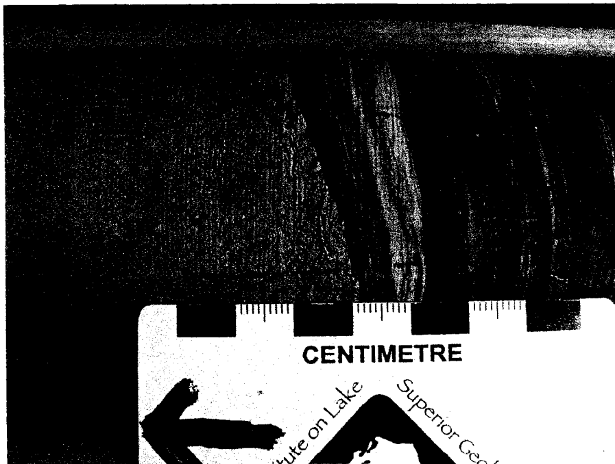
Fig.49 Distal Bar. Dewatering feature. Clay injections in the base of a sandstone layer probably formed during dewatering of the underlying flaser bedded sandstone to shale. Ripple laminated unit. Up is to the left. Core PR-98-3.
