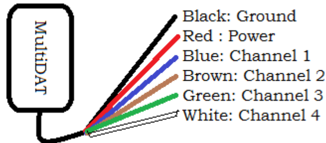
Figure 1. MultiDAT and connections.
