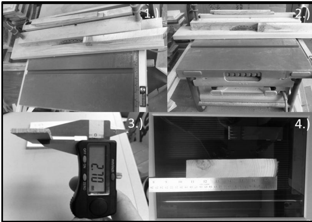
Figure 24. Ring width analysis sample preparation and analysis. 1.) “Swath” extracted from Disk – 00 for scanning, 2.) Sample being ran through LUWST X-Ray “jig”, 3.) Measuring thickness of sample prior to scanning, 4.) Ring width analysis specimen on scanner.
