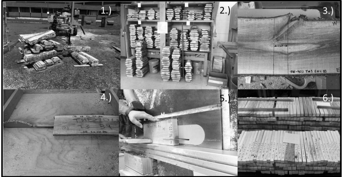
Figure 19. Mechanical and Physical Properties Specimen Preparation. 1.) Coarse refinement of bolts on Woodmizer-LT-40. 2.) Samples reducing in moisture content. 3.) Extraction of defects. 4.) Cutting slab in half on LUWSTF jig. 5.) Extracting radial positions from slabs. 6.) Stacked MOE / MOR samples in LUWSTF.
