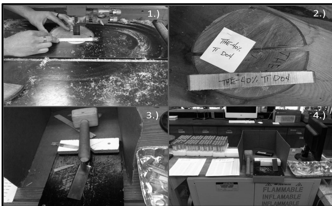
Figure 22.2 F.Q.A. Sample Preparation. 1.) Extracting 2 cm “swath” extending through the pith from bark to bark on band saw, 2.) “Cookie” processed into fiber specimen, 3.) Microtone and mallet processing station, 4.) Test tubes and processing station for FQA.
