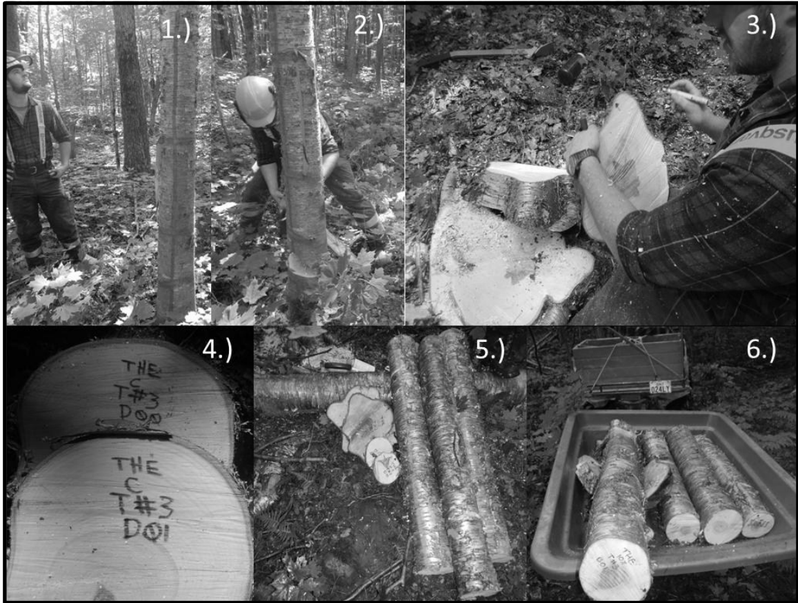
Figure 17. Field collection crew (Tyler Power) felling trees and processing specimens. 1.) Assessing standing crop tree (North direction on tree as red vertical line), 2.) Felling crop tree, 3.) Labelling crop tree in field, 4.) Labeled disks / cookies, 5.) Bolts and disks / cookies in field, 6.) Sample extraction via Quad Runner and wagon provided by Mr. Keith Hobak and LUWSTF.
