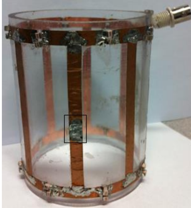
Figure 3.2: The 8 rung high pass birdcage resonator used for MRI (also showing a construction defect)
