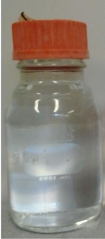
Figure 3.9 : Saline phantom used for MRI
