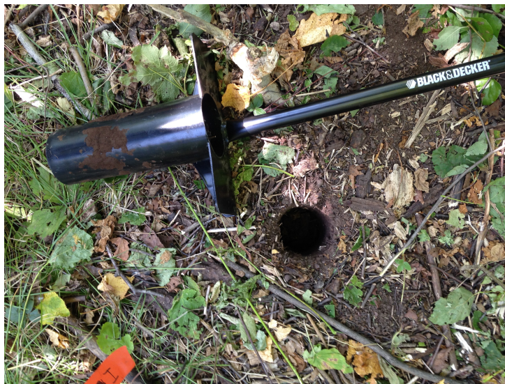
Figure 3.9. Bulb planting tool used to procure soil sample cores
