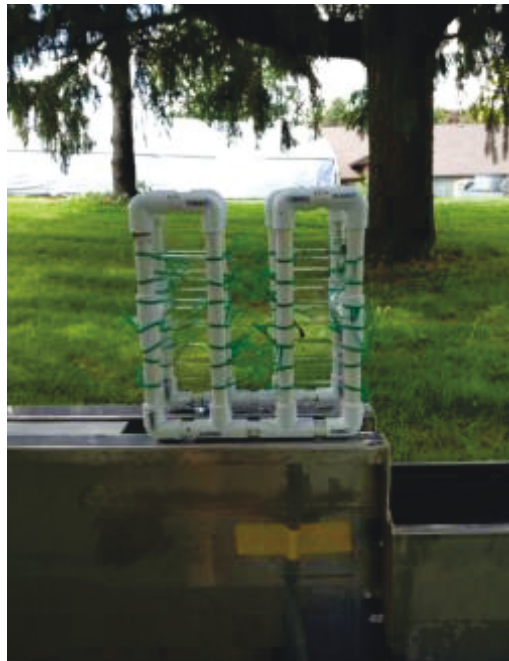
Figure 10: Photograph of the PVC rig holding slides.
