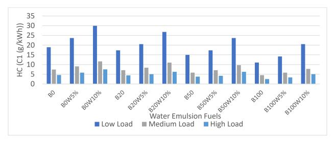
Figure 48: HC Emission of a Light-Duty Engine at Different Loads at 2100 rpm when Operated with Water Emulsion Fuel
