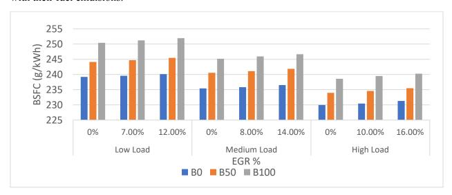
Figure 54: BSFC of a Light-Duty Engine at Different Loads with their EGR % at 2100 rpm
