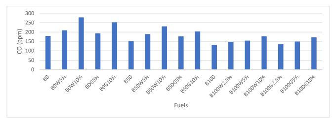
Figure 30: CO Emission in Heavy-Duty Engine at 1000 rpm
