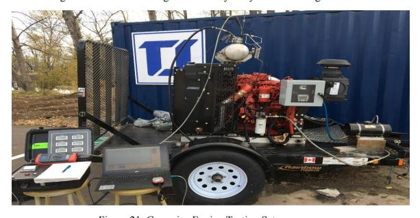
Figure 21: Cummins Engine Testing Setup
