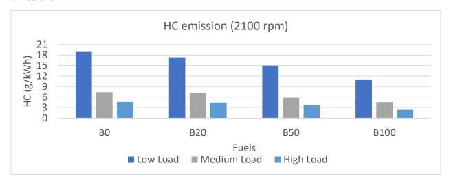
Figure 37: HC Emission of a Light-Duty Engine at Different Loads at 2100 rpm
