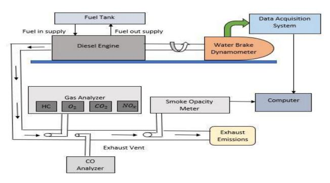
Figure 22: Schematic Diagram of HATZ Engine
