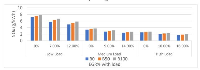
Figure 60: NOx Emission of a Light-Duty Engine at Different Loads with their EGR % at 2100 rpm
