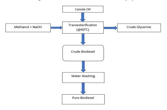
Figure 6: Steps to Produce Biodiesel
