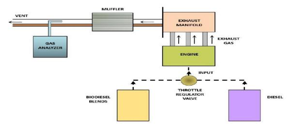
Figure 20: Schematic Diagram of Heavy-Duty Cummins Engine
