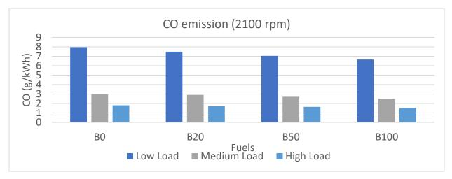
Figure 36: CO Emission of a Light-Duty Engine at Different Loads at 2100 rpm
