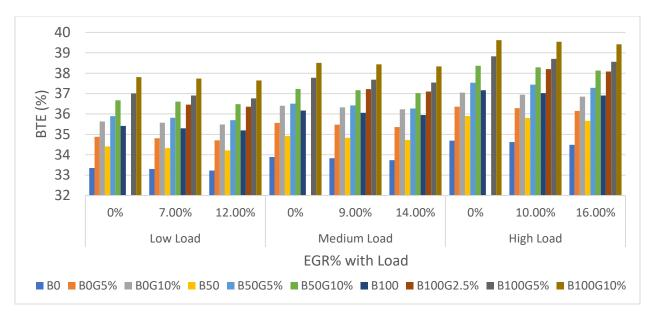
Figure 59: BTE of a Light-Duty Engine at Different Loads with their EGR% at 2100 rpm when Operated with Glycerine Emulsion Fuel
