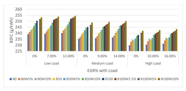
Figure 55: BSFC of a Light-Duty Engine at Different Loads with their EGR% at 2100 rpm when Operated with Water Emulsion Fuel
