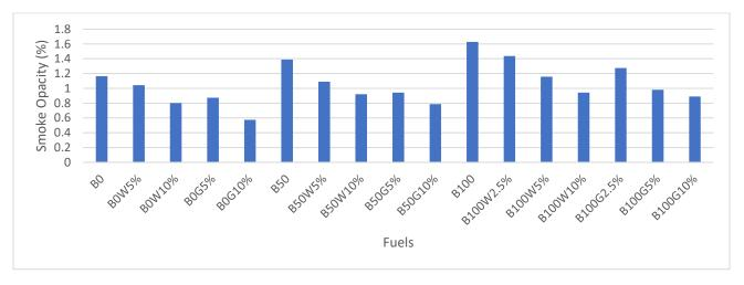
Figure 32: Smoke Opacity Emission in Heavy-Duty Engine at 1000 rpm
