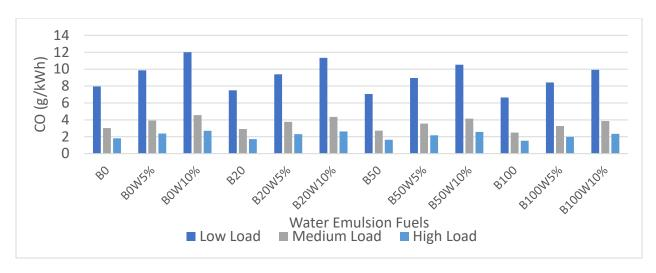
Figure 46: CO Emission of a Light-Duty Engine at Different Loads at 2100 rpm when Operated with Water Emulsion Fuel
