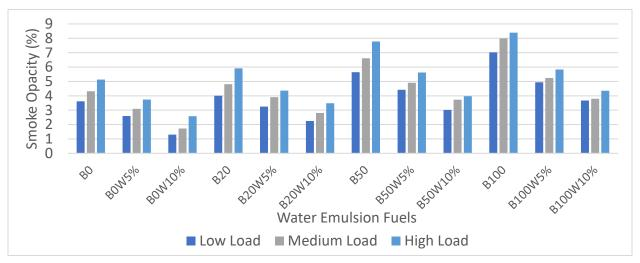
Figure 50: Smoke Opacity of a Light-Duty Engine at Different Loads at 2100 rpm when Operated with Water Emulsion Fuel
