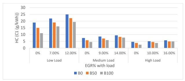
Figure 66: HC Emission of a Light-Duty Engine at Different Loads with their EGR % at 2100 rpm
