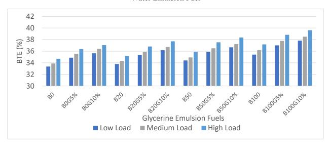
Figure 43: BTE of a Light-duty Engine at Different Loads at 2100 rpm when Operated with Glycerine Emulsion Fuel
