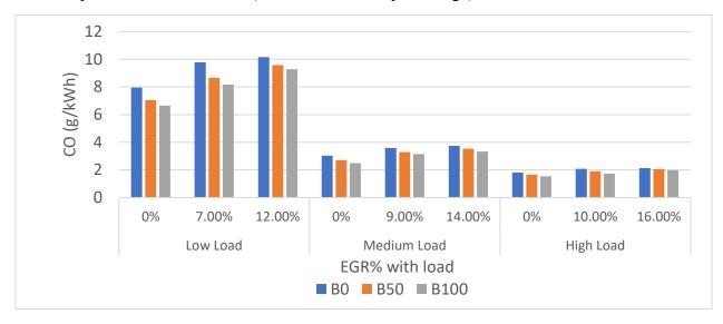
Figure 63: CO Emission of a Light-Duty Engine at Different Loads with their EGR % at 2100 rpm
