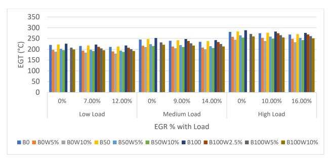
Figure 73: EGT of a Light-Duty Engine at Different Loads with their EGR% at 2100 rpm when Operated with Water Emulsion Fuel
