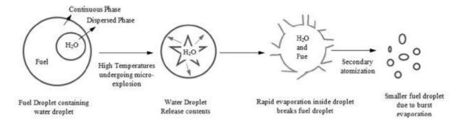
Figure 3: Atomization with Micro-Explosion [71]
