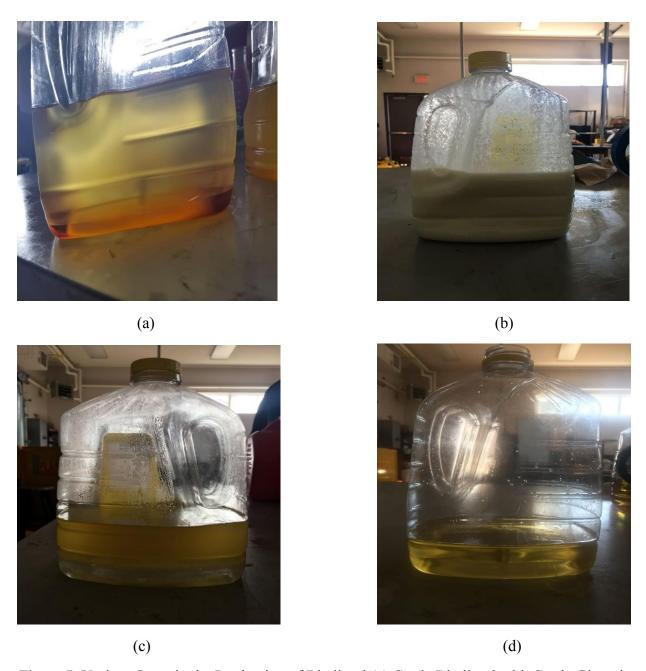
Figure 7: Various Steps in the Production of Biodiesel (a) Crude Biodiesel with Crude Glycerine (b) Biodiesel on First Wash (c) Separation after Second Wash (d) Pure Biodiesel
