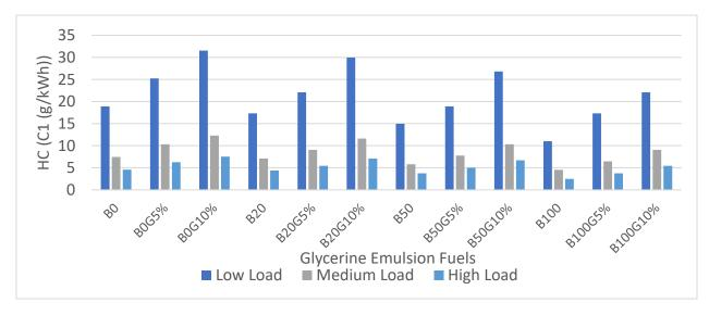
Figure 49: HC Emission of a Light-Duty Engine at Different Loads at 2100 rpm when Operated with Glycerine Emulsion Fuel
