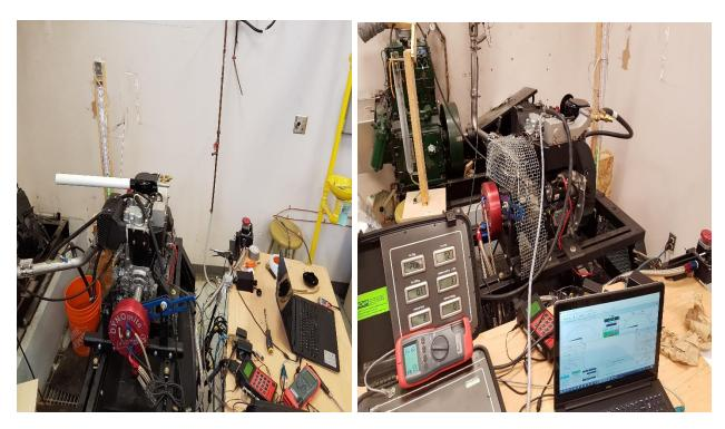
Figure 23: HATZ (Light duty) Engine Test Setup
