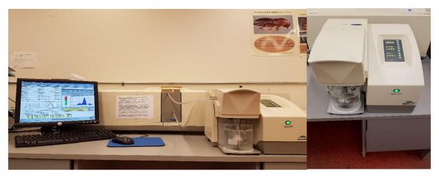
Figure 16: Malvern Mastersizer Hydro 2000S to measure the droplet size of the particle
