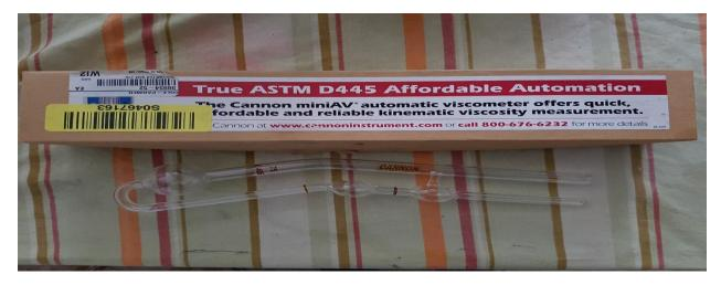
Figure 13: Kinematic Viscometer
