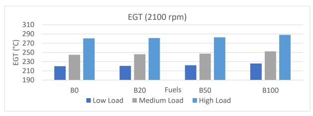
Figure 39: EGT of a Light-Duty Engine at Different Loads at 2100 rpm
