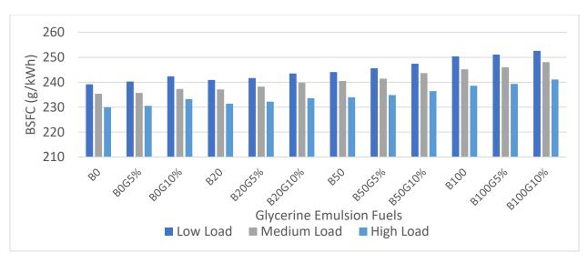
Figure 41: BSFC of a Light-Duty Engine at Different Loads at 2100 rpm when Operated with Glycerine Emulsion Fuel
