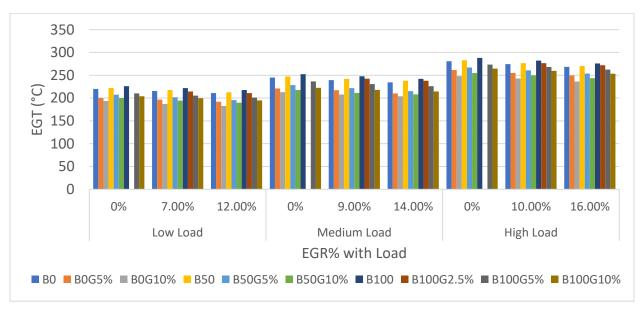
Figure 74: EGT of a Light-Duty Engine at Different Loads with their EGR% at 2100 rpm when Operated with Glycerine Emulsion Fuel
