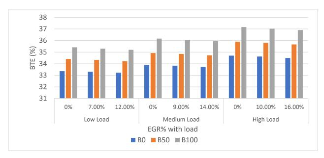
Figure 57: BTE of a Light-Duty Engine at Different Loads with their EGR % at 2100 rpm
