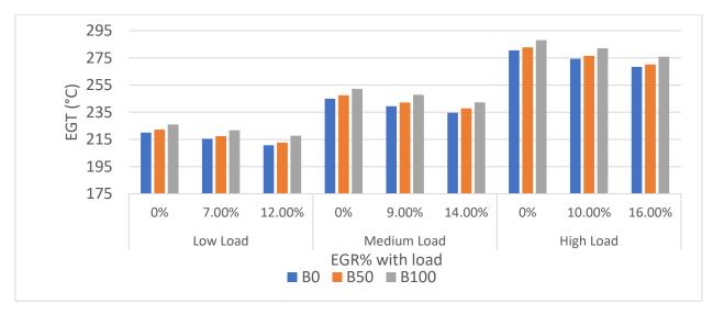
Figure 72: EGT of a Light-Duty Engine at Different Loads with their EGR % at 2100 rpm
