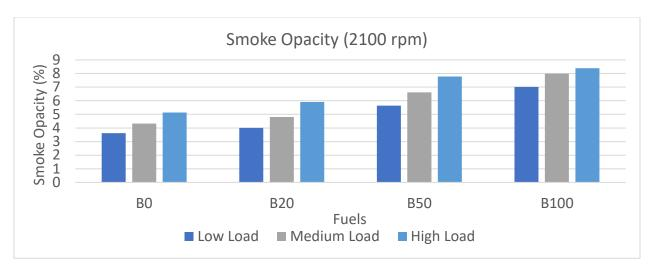
Figure 38: Smoke Opacity of a Light-Duty Engine at Different Loads at 2100 rpm
