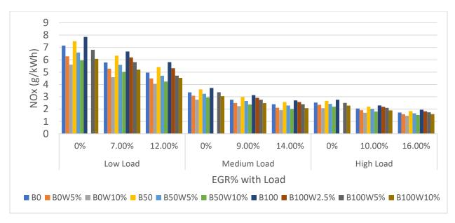
Figure 61: NOx Emission of a Light-Duty Engine at Different Loads with their EGR% at 2100 rpm when Operated with Water Emulsion Fuel
