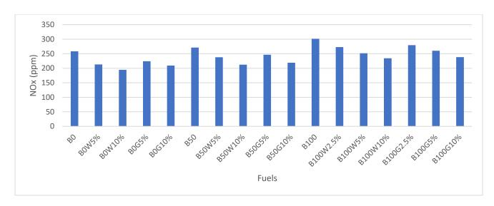
Figure 29: NOx Emission in Heavy-Duty Engine at 1000 rpm
