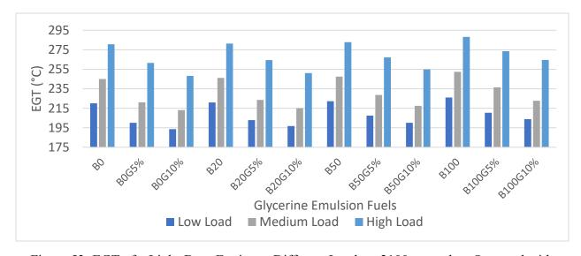
Figure 53: EGT of a Light-Duty Engine at Different Loads at 2100 rpm when Operated with Glycerine Emulsion Fuel
