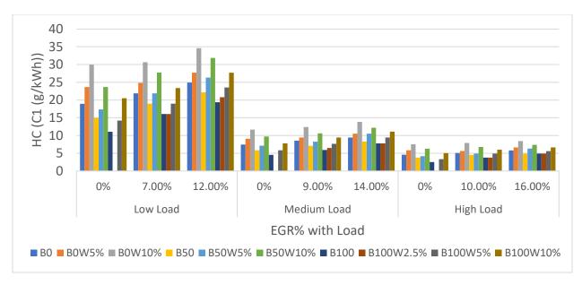
Figure 67: HC Emission of a Light-Duty Engine at Different Loads with their EGR% at 2100 rpm when Operated with Water Emulsion Fuel
