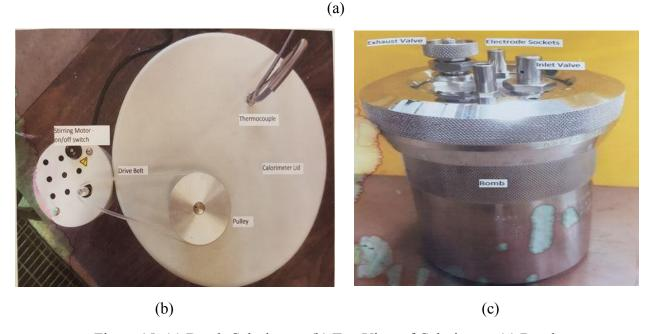
Figure 15: (a) Bomb Calorimeter (b) Top View of Calorimeter (c) Bomb
