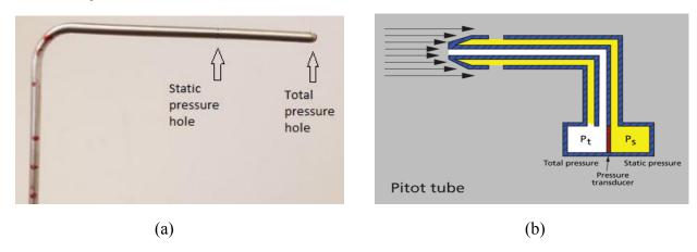
Figure 18: (a) Marking of two different pressure collecting points (b) Diagram of Pitot Tube
