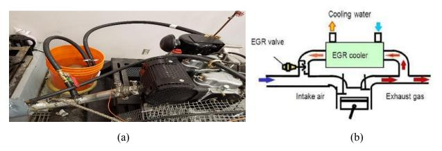
Figure 4: (a) Pictorial and (b) Schematic Working [108] of the EGR System
