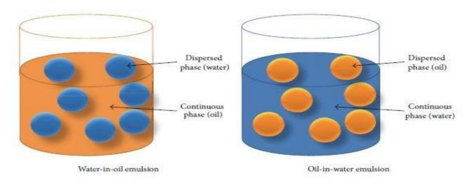
Figure 11: Pictorial View of the Two-Phase Emulsion [119]
