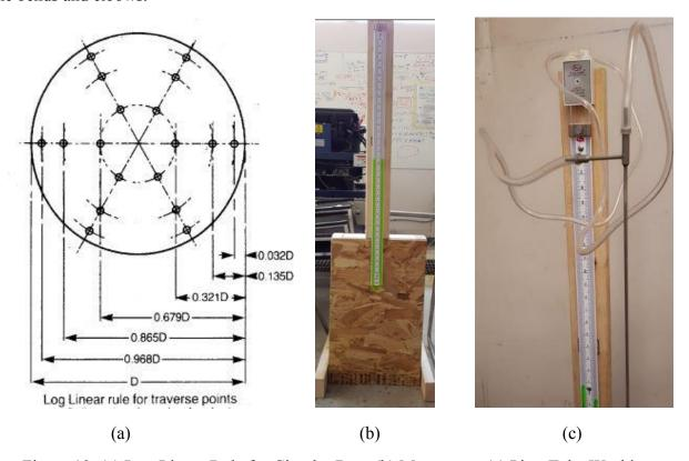
Figure 19: (a) Log-Linear Rule for Circular Duct (b) Manometer (c) Pitot Tube Working
