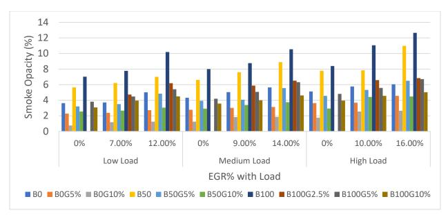
Figure 71: Smoke Opacity of a Light-Duty Engine at Different Loads with their EGR% at 2100 rpm when Operated with Glycerine Emulsion Fuel
