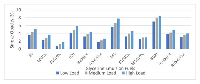
Figure 51: Smoke Opacity of a Light-Duty Engine at Different Loads at 2100 rpm when Operated with Glycerine Emulsion Fuel
