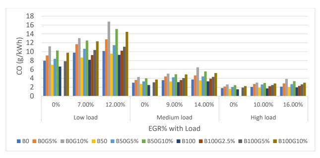
Figure 65: CO Emission of a Light-Duty Engine at Different Loads with their EGR% at 2100 rpm when Operated with Glycerine Emulsion Fuel
