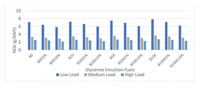
Figure 45: NOx Emission of a Light-Duty Engine at Different Loads at 2100 rpm when Operated with Glycerine Emulsion Fuel
