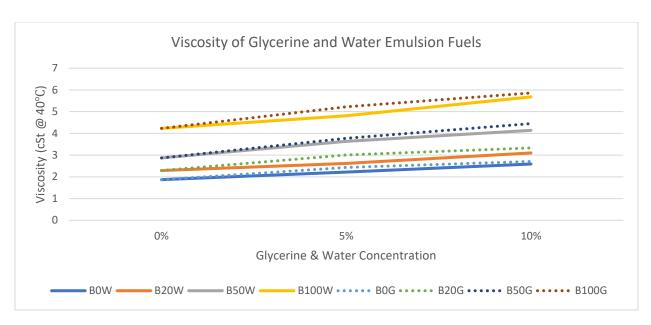
Figure 27: Kinematic Viscosity of Emulsion Fuels
