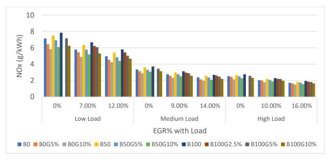
Figure 62: NOx Emission of a Light-Duty Engine at Different Loads with their EGR% at 2100 rpm when Operated with Glycerine Emulsion Fuel
