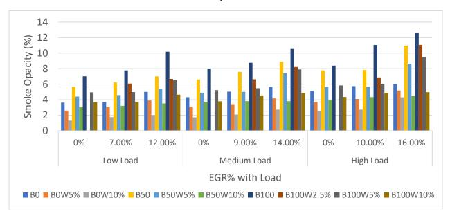
Figure 70: Smoke Opacity of a Light-Duty Engine at Different Loads with their EGR% at 2100 rpm when Operated with Water Emulsion Fuel
