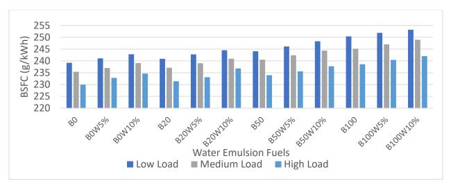
Figure 40: BSFC of a Light-Duty Engine at Different Loads at 2100 rpm when Operated with Water Emulsion Fuel
