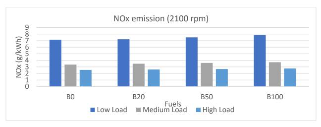
Figure 35: NOx Emission of a Light-Duty Engine at Different Loads 2100 rpm
