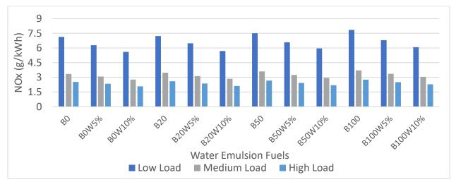
Figure 44: NOx Emission of a Light-Duty Engine at Different Loads at 2100 rpm when Operated with Water Emulsion Fuel
