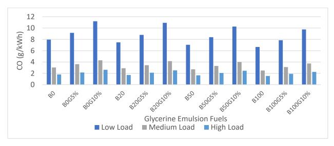
Figure 47: CO Emission of a Light-Duty Engine at Different Loads at 2100 rpm when Operated with Glycerine Emulsion Fuel
