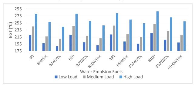
Figure 52: EGT of a Light-Duty Engine at Different Loads at 2100 rpm when Operated with Water Emulsion Fuel
