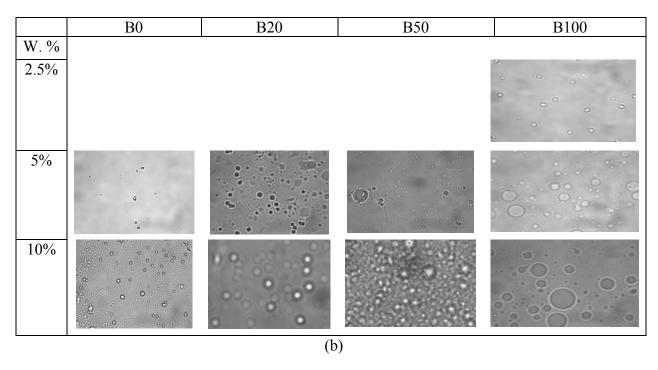
Figure 26: (a) Bimodal Particle Size Distribution Graphs and (b) Microscopic Pictures of the Water Emulsion Fuels
