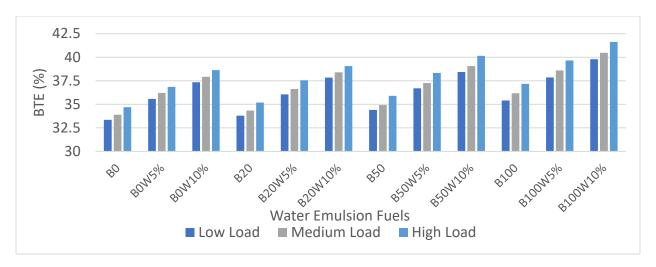
Figure 42: BTE of a Light-Duty Engine at Different Loads at 2100 rpm when Operated with Water Emulsion Fuel
