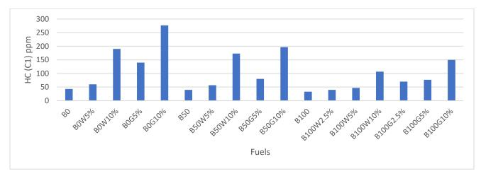
Figure 31: HC Emission in Heavy-Duty Engine at 1000 rpm
