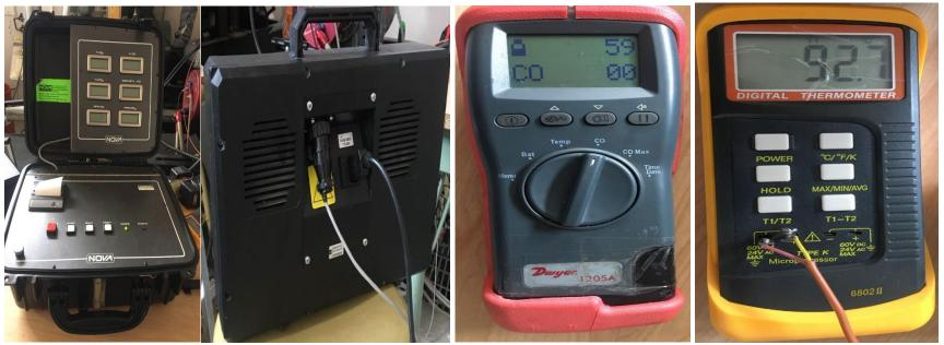
Gas Analyzer Smoke Opacity Meter CO Analyzer Thermometer
