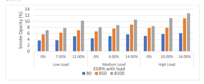
Figure 69: Smoke Opacity of a Light-Duty Engine at Different Loads with their EGR % at 2100 rpm
