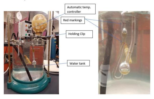
Figure 12: Setup for the Viscosity Test
