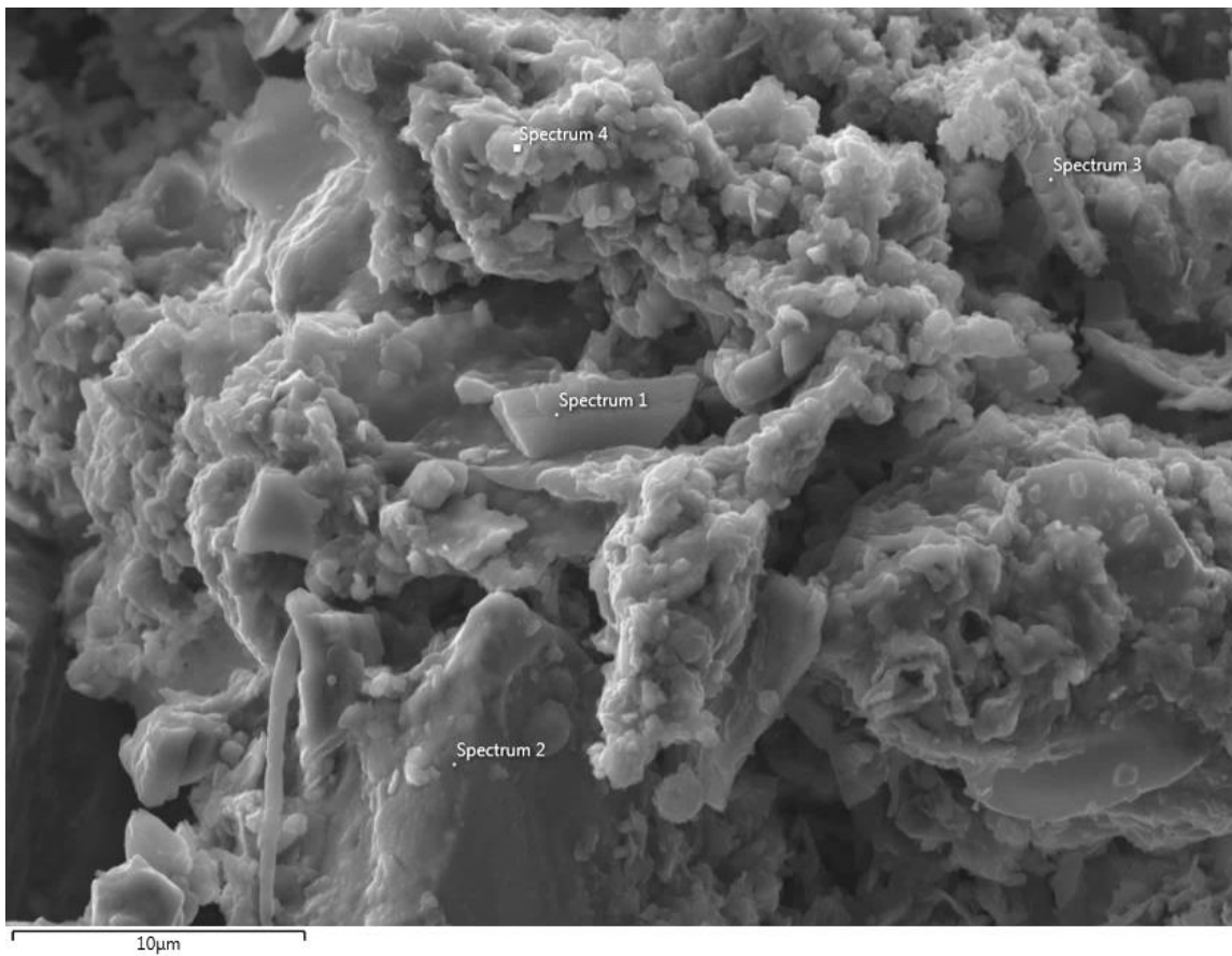
Figure 6.24: Secondary electron image of sample 2C showing quartz and silicate grains of the silica sand and creek sediment.
