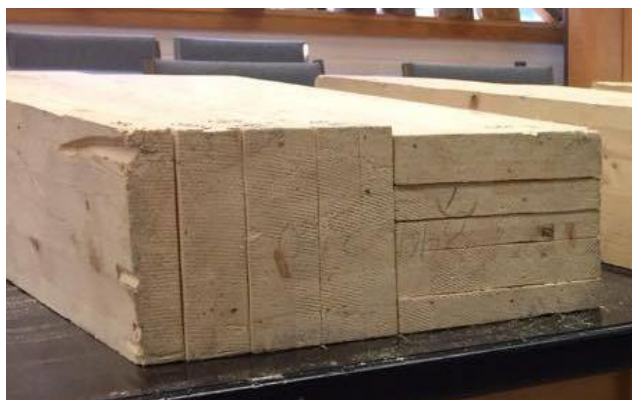
Figure 1. A glulam bolt that has been cut in half then the boards cut from the two different orientations, parallel and perpendicular.
