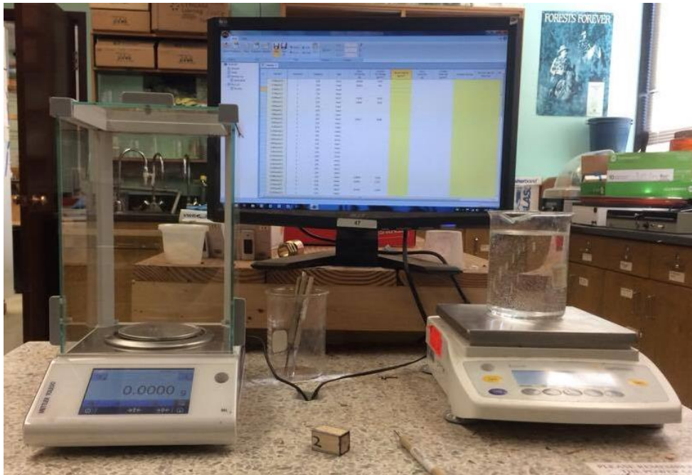
Figure 2. Scale for measuring the mass of the density samples and the scale and beaker combination for measuring the volume of the density samples.
