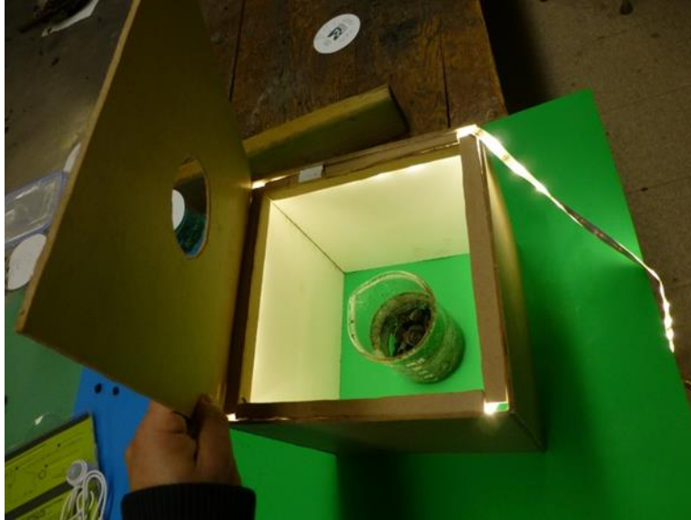
Figure 13: The illumination box placed on the top of a sample
