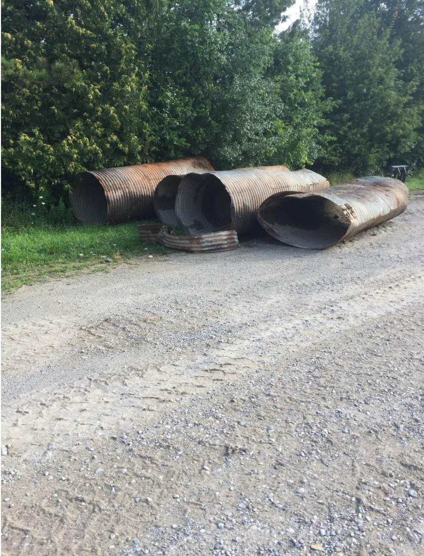
Figure 5. view of metal culverts (Ewaskiw 2017)
