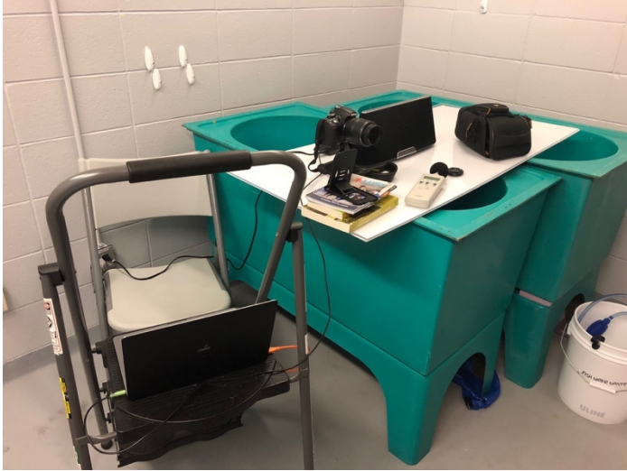
Figure A 2 Set up used to capture fish reactions. Included a MacBook, DSLR, speaker, sound reading device and an iPhone.
