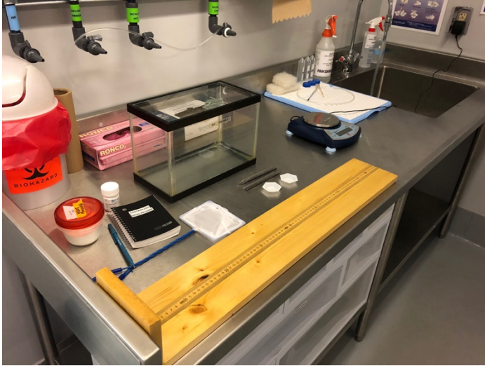
Figure A 4 Set up used to measure length and weight of the study fish
