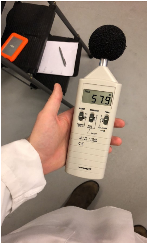
Figure A 3 Sound measuring device used to test decibel readings during tests
