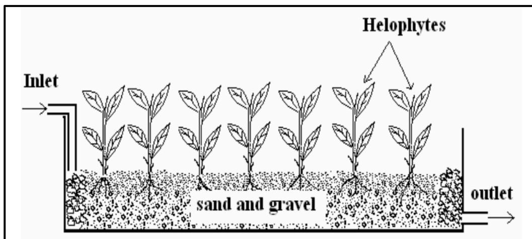
Figure 2. Design of a Subsurface Flow Constructed Wetland
