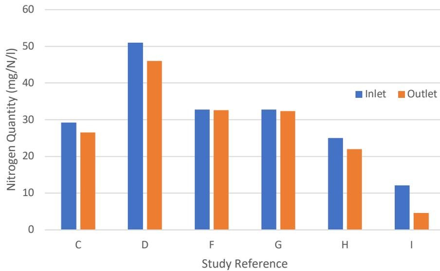
Figure 5. Inlet and outlet quantity of nitrogen in each constructed wetland designed for plant assimilation
