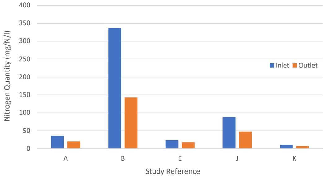
Figure 3. Inlet and outlet quantity of nitrogen for each constructed wetland designed for denitrification / nitrification removal
