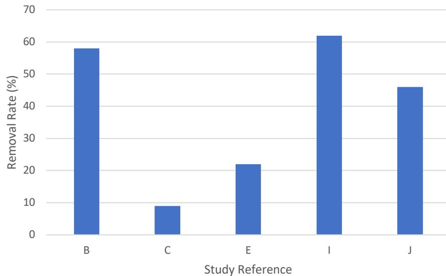
Figure 10. Nitrogen removal rates for each corresponding subsurface flow constructed wetland
