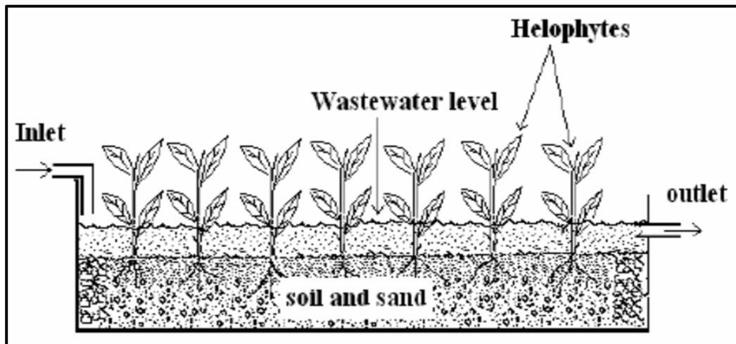
Figure 1. Design of a Surface Flow Constructed Wetland
