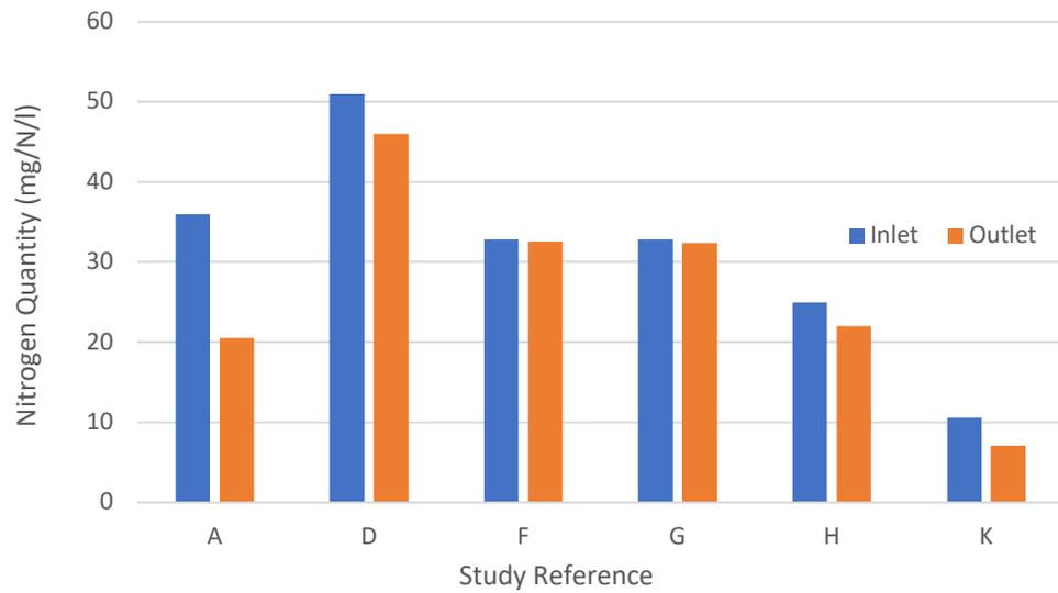
Figure 7. Inlet and outlet quantity of nitrogen within each surface flow constructed wetland
