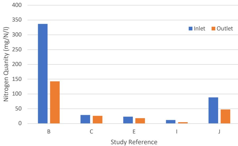
Figure 9. Inlet and outlet quantity of nitrogen within each subsurface flow constructed wetland
