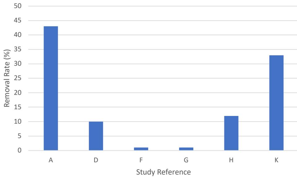
Figure 8. Nitrogen removal rates for each corresponding surface flow constructed wetland
