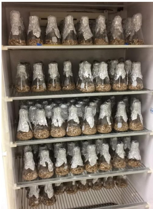
Figure 7. 150 Erlenmeyer flasks in incubator for incubation at 20°C
