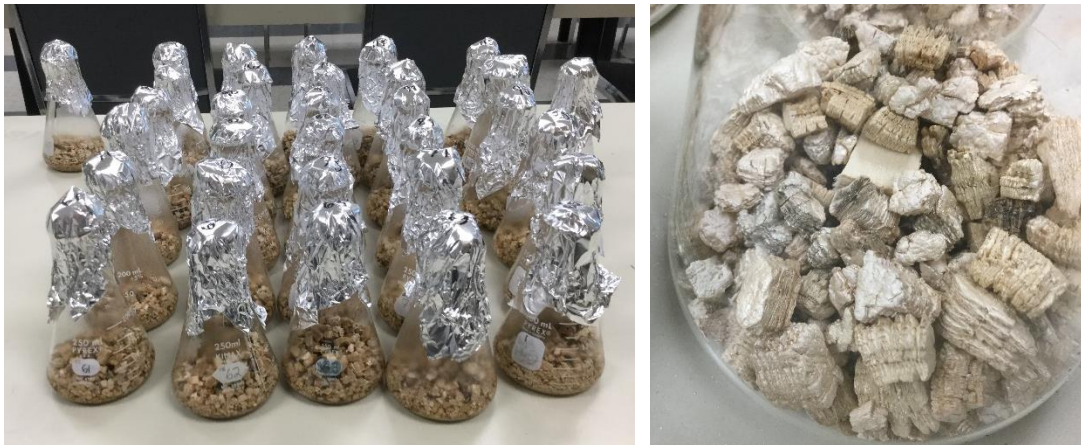
Figure 3. Flasks prepared with vermiculite-peat mixture and malt extract broth before being autoclaved.
