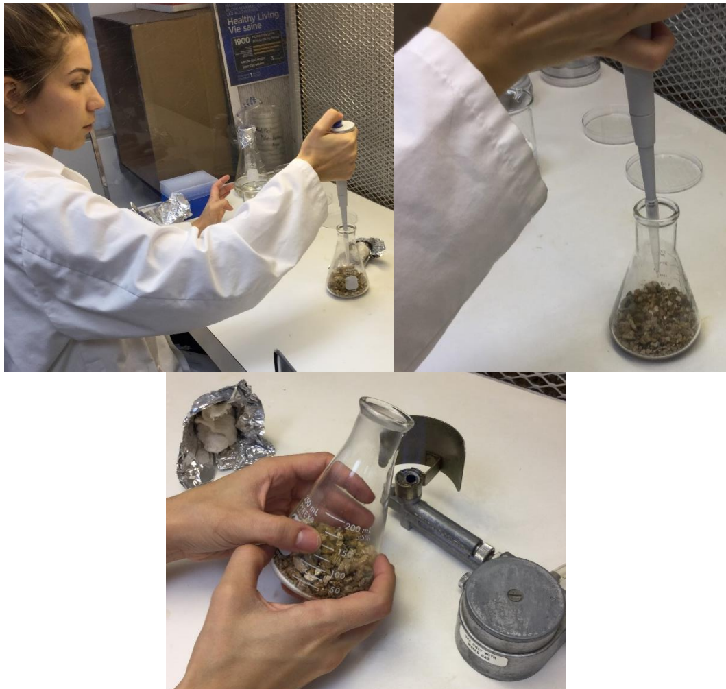
Figure 6. Author using Eppendorf micropipette to inoculate 200 nematodes/mL of Aphelenchoides sp. (top) and sterilize flask using Bunsen burner (bottom).
