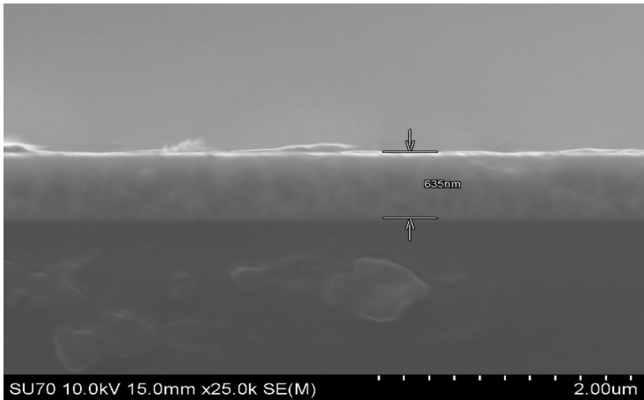
Figure 32: Cross sectional view of SEM result of sample 5 with film thickness measurement
