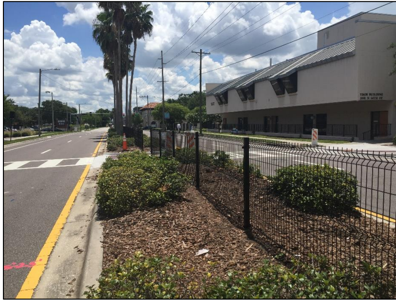
Figure 6.27: Median fencing to channelize pedestrians into marked crosswalks (City of Tampa, 2017).
