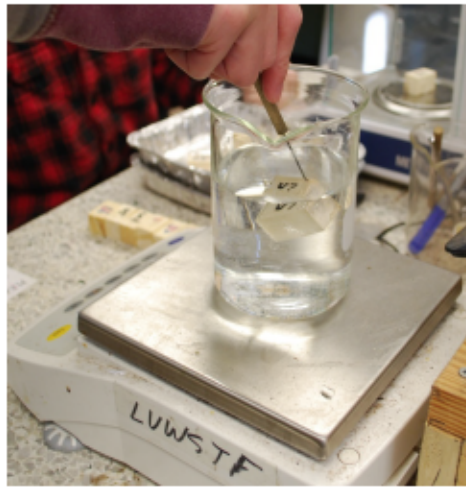
Figure 16. An illustration of the water displacement method to obtain density.
