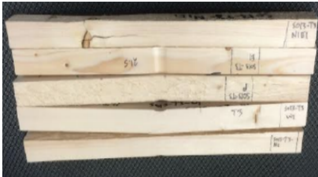
Figure. 15. The specimens after the MOE testing with density cubes marked.
