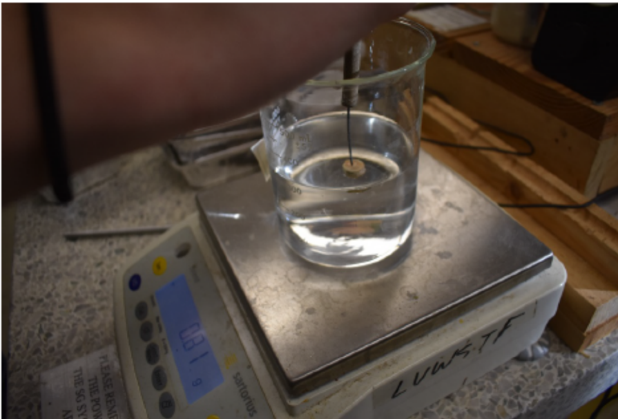
Figure 5: Volume of sectioned sample measured using water displacement technique.
