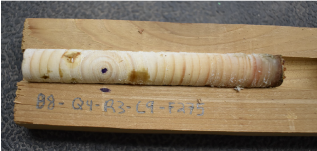
Figure 3: Collected sampled mounted to wooden trough and labeled.
