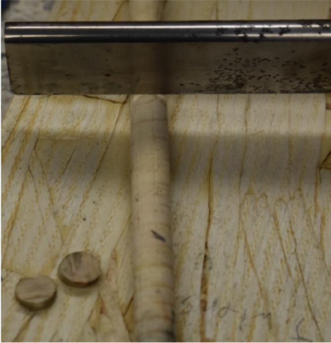
Figure 4: Sample sectioned in 5 ring increment from pith.
