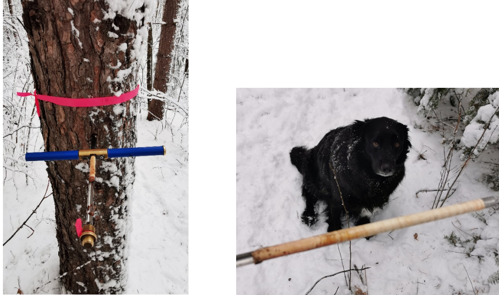
Figure 3 Pinus resinosa core extraction using an increment borer (left). Extracted core in spoon (right).
