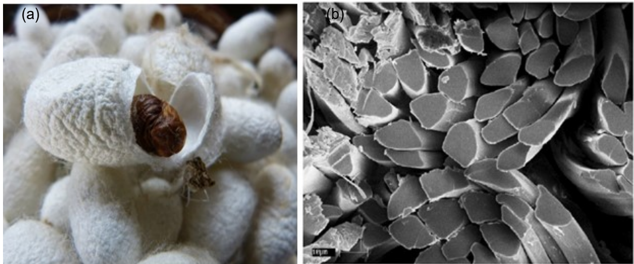
Figure 2.10: Silk fiber-Silk cocoon (a)(source: www.materialdistrict.com ), cross sectional view (b)
