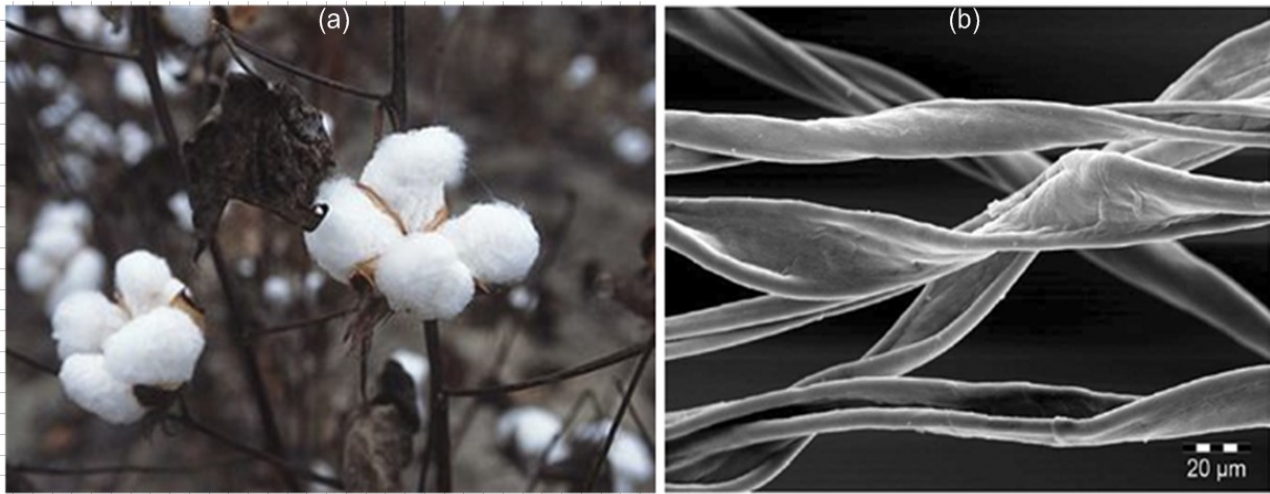
Figure 2.12: Cotton seed (a) and longitudinal view of cotton fibers (b) [5, 44]
