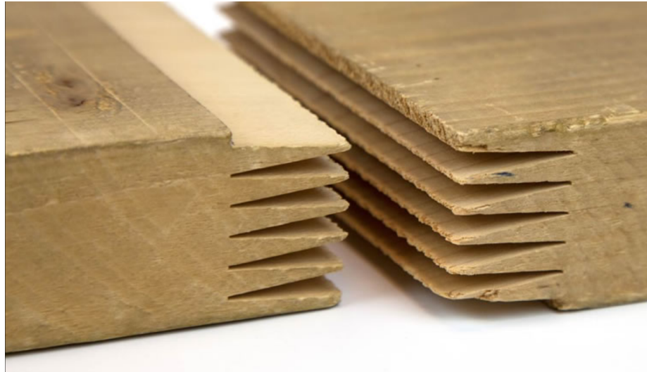
Figure 14. A common finger joint before it is glued and pressed together. Note the significant amount of surface area for gluing (Government of Canada 2020c).
