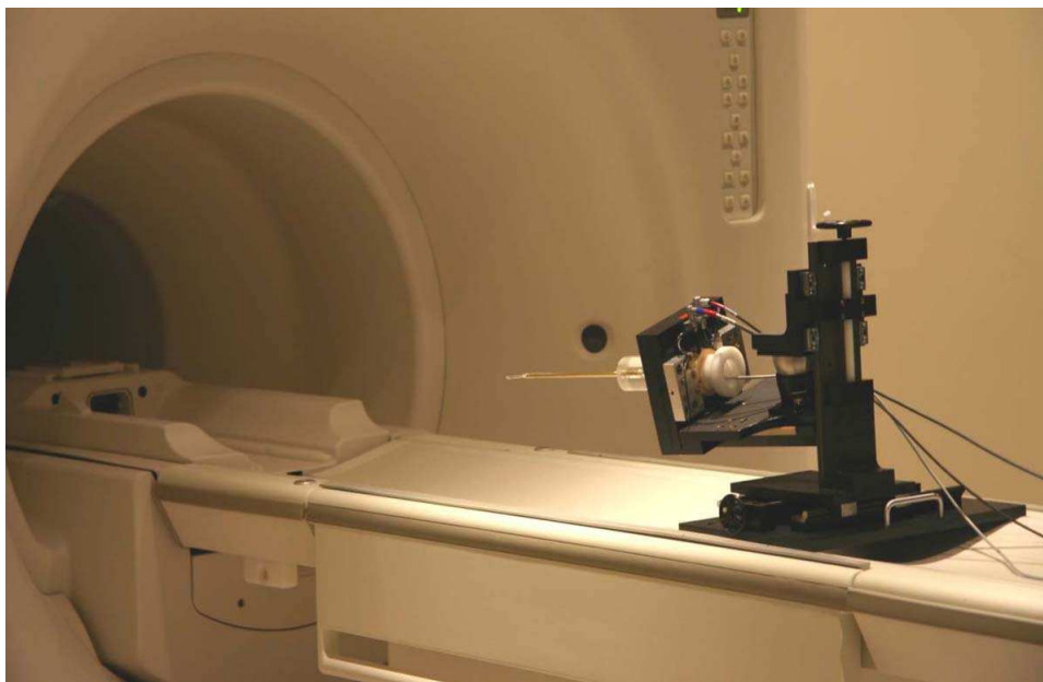
Figure 2.5: MRI-compatible positioning system and rotational motor attached to the heating applicator (Chopra et al. 2008).
