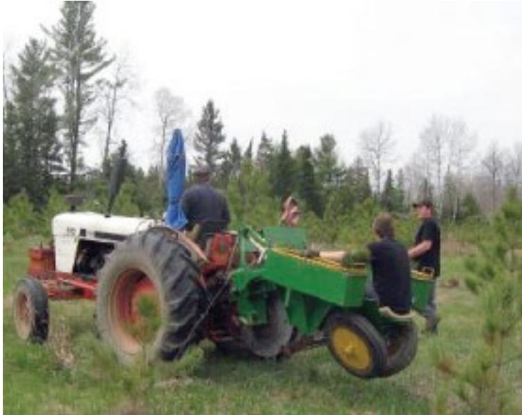
Figure 9 - An example of a planting machine towed behind a small farm tractor (OMNRF 2019)
