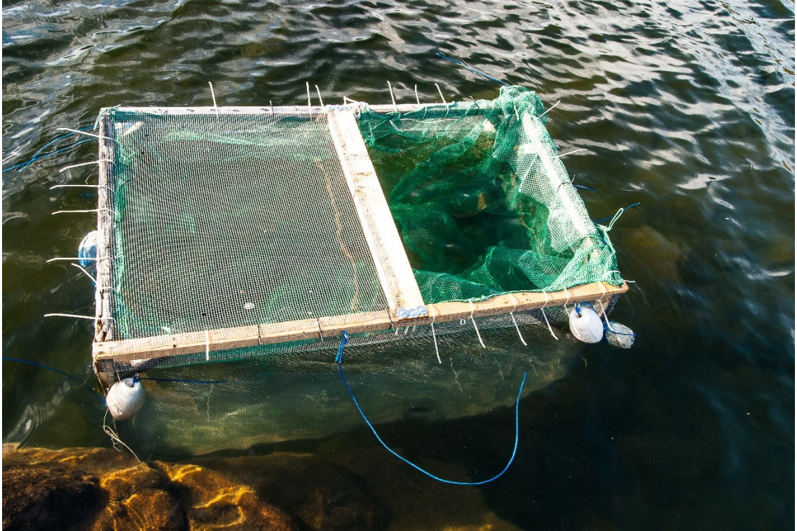
Figure A3: Image of submerged fish pens (0.91 m x 1.52 m x 0.91m) composed of a mesh bag with 4mm holes surrounded by a galvanized steel cage with 5 mm square holes and a 1 mm thick wire, used for temporary housing of fish used in the experiments.
