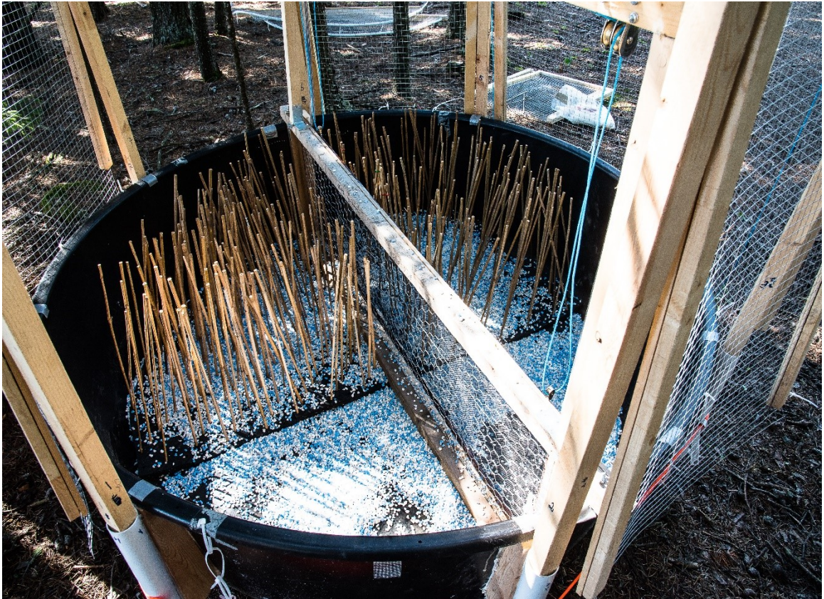
Figure A1: Image of one of the experimental enclosures used in the experiment (before water was added showing the gravel used to provide contrast for visual recordings and the bamboo cover plates on either side of the central gate and barrier to provide cover for Yellow Perch.
