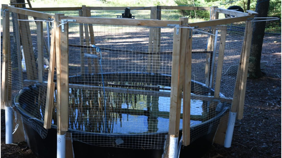
Figure A2: Image of one of the experimental enclosures filled with water. The perimeter fence of the enclosure was composed of 8 wooden panels zip-tied to support posts and the lip of the tub. The roof (not shown) was made from two half-moon shaped panels that rested on top of the support posts. Remotely activated video recorders are attached to the centre wooden frame that supports the moveable mesh gate that is used to restrict movement between the halves of the enclosure.
