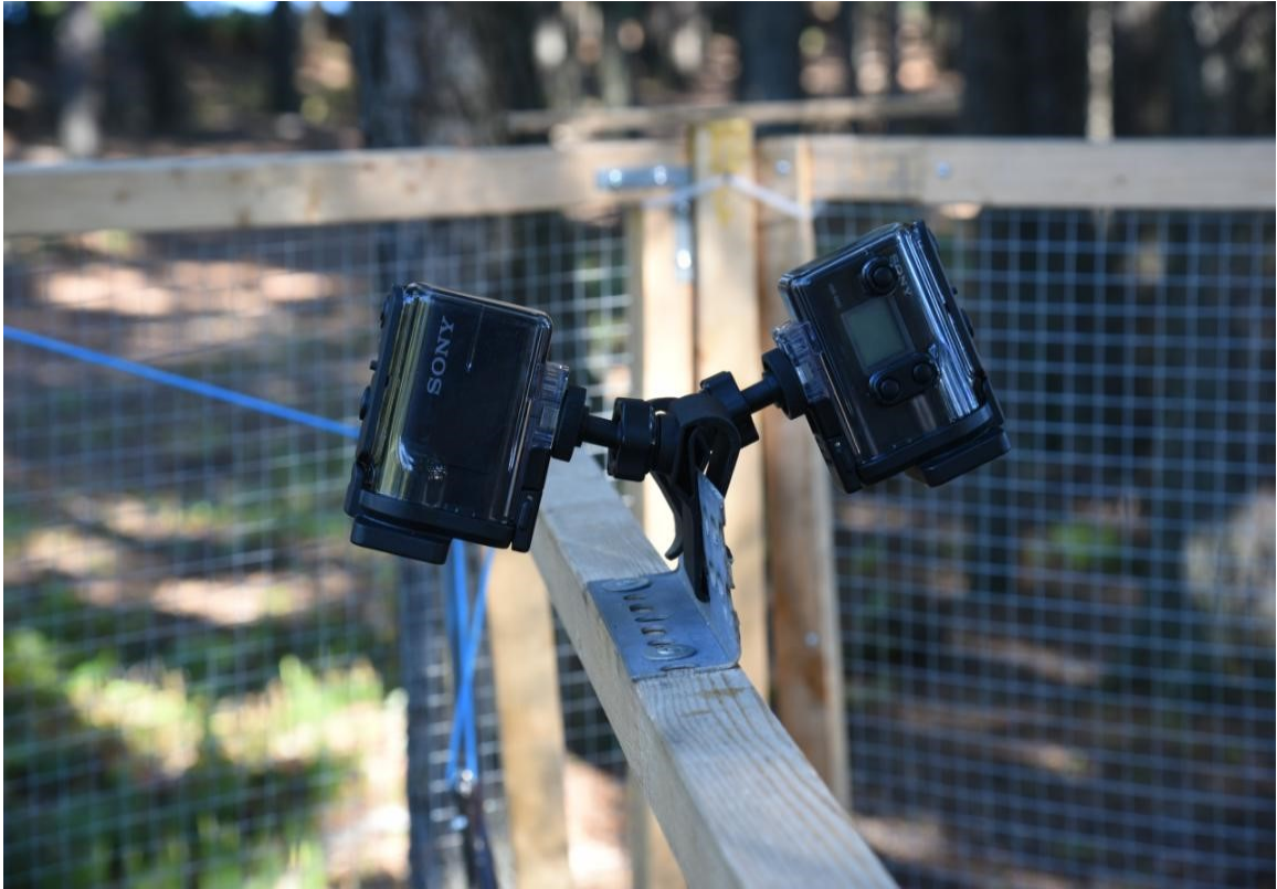
Figure A7: Image of the remotely activated video recorders that were mounted on a bracket above the centre of the enclosure. Each camera viewed one half of the enclosure. Images from the enclosure were processed and the data intergrated for each enclosure and trial of the experiment.
