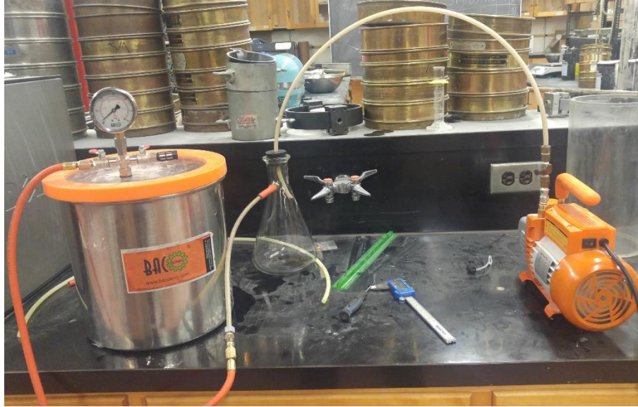
Figure 3.1: The vacuum pump system used in resaturation.
